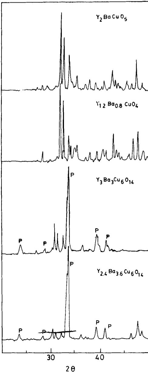
**Figure 2.** X-ray powder patterns of  $\text{Y}_{3-x}\text{Ba}_{3+x}\text{Cu}_6\text{O}_{14}$ ,  $\text{Y}_2\text{BaCuO}_5$  and  $\text{Y}_{1.2}\text{Ba}_{0.8}\text{CuO}_4$ .
