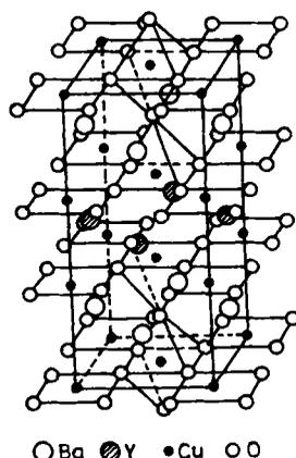
**Figure 1.** Proposed structure of  $\text{Y}_2\text{Ba}_4\text{Cu}_6\text{O}_{14\pm\delta}$  analogous to  $\text{La}_3\text{Ba}_3\text{Cu}_6\text{O}_{14}$  (following Er-Rakho *et al* 1981).  $A_1$  and  $A_2$  sites are shown. Y occupies  $A_2$  sites preferentially.
