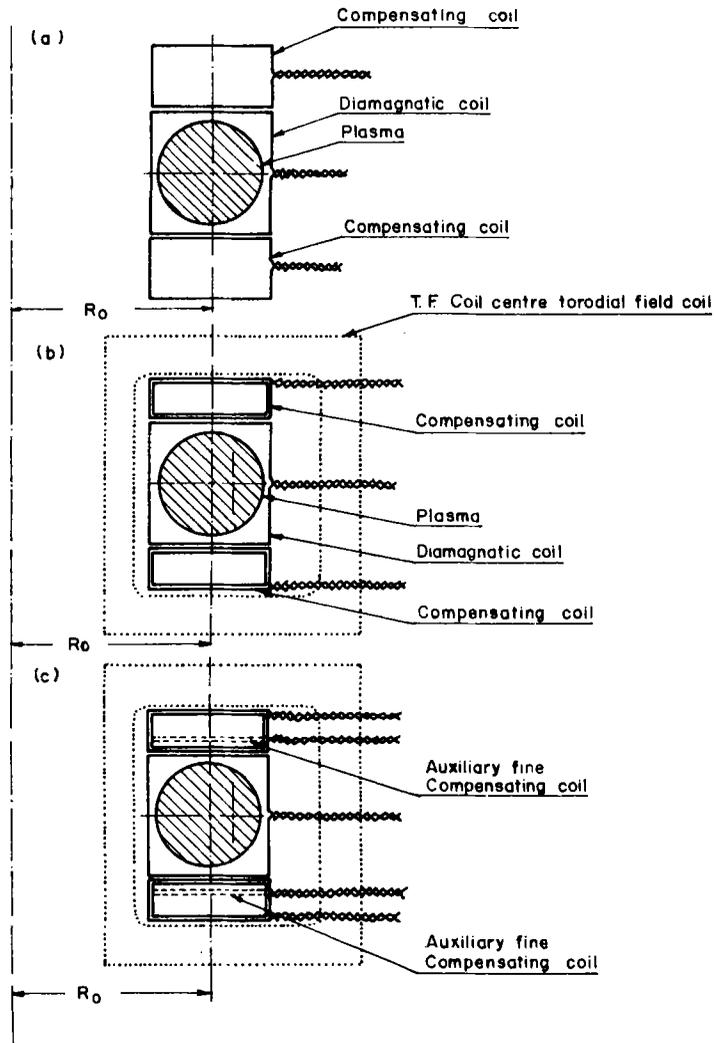
**Figure 2.** Schematics of measuring plasma diamagnetism with a rectangular coil compensated by (a) two one-turn non-encircling coils, (b) two two-turn non-encircling coils and (c) two two-turn non-encircling coils and an auxiliary coil for initial external fine adjustment. The dashed lines indicate the dimensions of toroidal field coils of Aditya.
