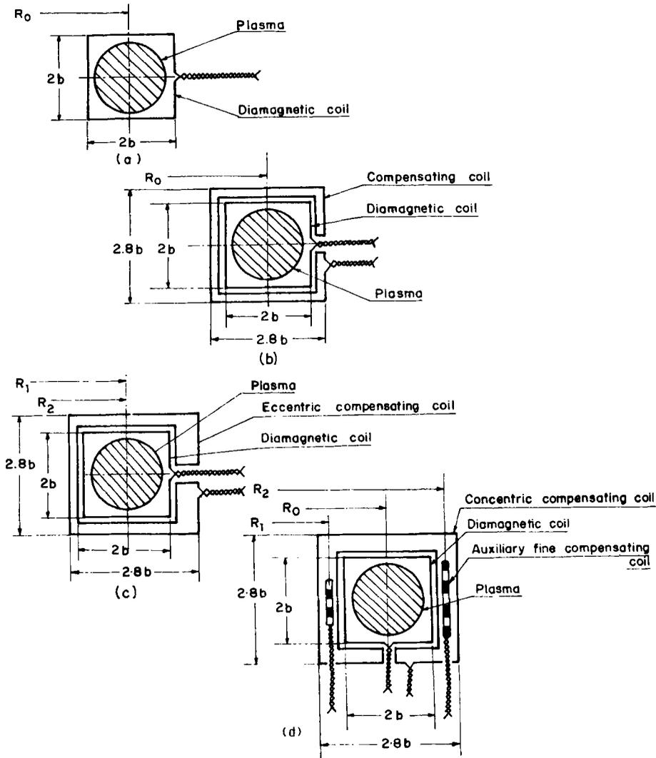
**Figure 1.** Schematics of measuring plasma diamagnetism with (a) a single turn rectangular coil, (b) concentric diamagnetic and compensating coil, (c) eccentric coil system and (d) auxiliary coils for external fine compensation adjustment and fine eccentricity adjustment.
