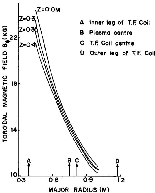
Figure 3. Toroidal magnetic field due to toroidal field coils on Aditya varies as a function of  $R$  for different values of  $Z$ .
