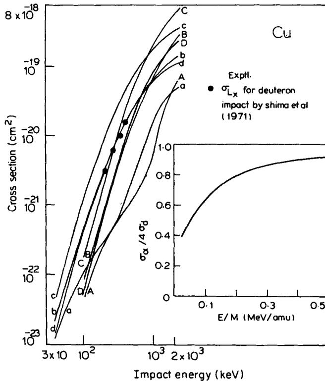
**Figure 2.** Cross-sections of Cu. Curves A and a: Same as in figure 1; Curves B and C: Present values of  $\sigma_{L_I} + \sigma_{L_{II}}$  and  $\sigma_L$  respectively; Curve D:  $10^2 \times \sigma_{LX}$  (present values); Curves b, c and d: Quantities (deuteron impact) corresponding to curves B, C, D.
