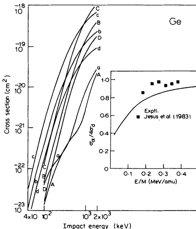
**Figure 3.** Cross-sections for Ge. Same as in figure 2 except Curves D and d:  $10 \times \sigma_{LX}$  for  $\text{He}^{2+}$  and deuteron impact respectively (present results).
