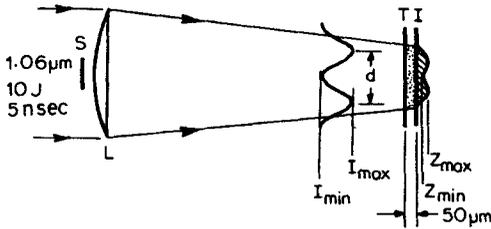
Figure 3. Schematic diagram to explain the meaning of  $I_{max}$ ,  $I_{min}$ ,  $Z_{max}$ ,  $Z_{min}$ -L-focusing lens; T, target foil; I, impact foil; S, strip.
