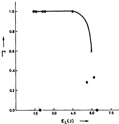
Figure 4. Variation of  $\Gamma$  with laser energy ( $E_L$ ). \* 10  $\mu\text{m}$  plastic,  $d = 75 \mu\text{m}$ ;  $\times$  10  $\mu\text{m}$  plastic,  $d = 150 \mu\text{m}$ ;  $\oplus$  10  $\mu\text{m}$  plastic with 0.1  $\mu\text{m}$  gold coating,  $d = 75 \mu\text{m}$ ;  $\#$  10  $\mu\text{m}$  plastic with 0.1  $\mu\text{m}$  gold coating,  $d = 150 \mu\text{m}$ . Incident laser intensity =  $2 \times 10^{11} \text{ W/cm}^2$  per joule.
