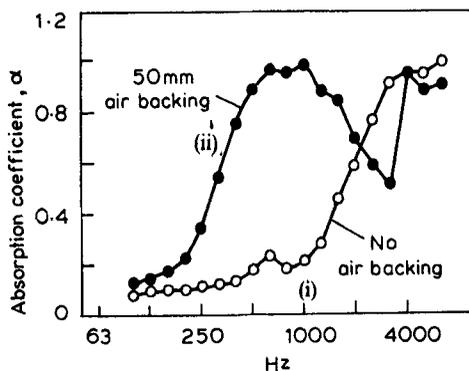
Figure 1. Sound absorption coefficient measured with standing wave tube.
