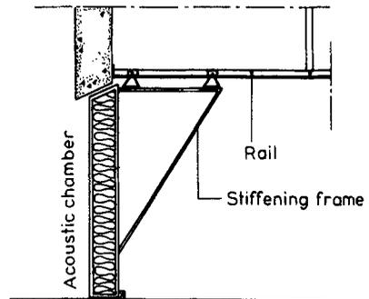
Figure 5. Door of acoustic chamber.
