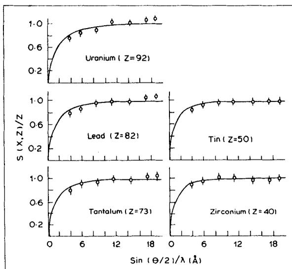
**Figure 3.** Variation of incoherent scattering function with momentum transfer of 279.2 keV photons by U, Pb, Ta, Sn and Zr. The lines indicate the theoretical values based on the non-relativistic HFS calculation values of Hubbell *et al* (1975). Circles represent experimental points.
