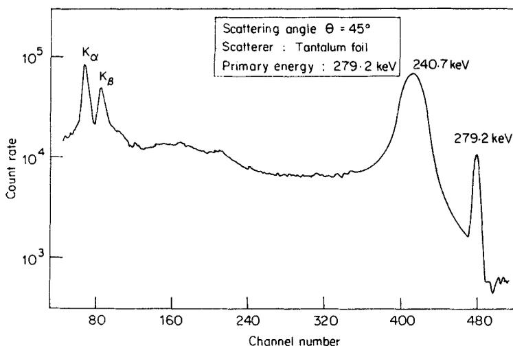
**Figure 2.** Scattered photon spectrum of primary energy 279.2 keV photons corresponding to 18 mg/cm<sup>2</sup> Ta scatterer at an angle 45°.
