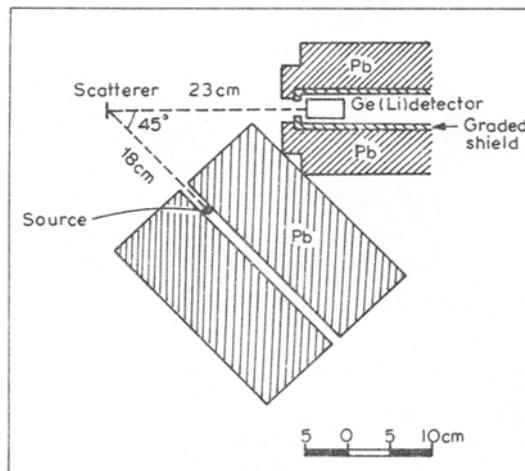
Figure 1. Experimental arrangement for measurement of scattered photons.
