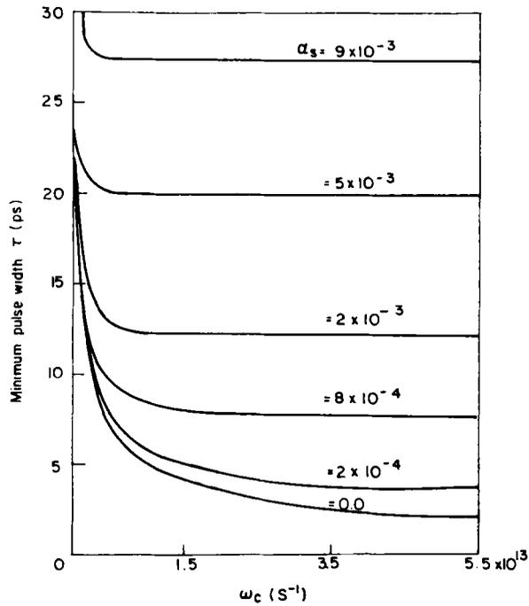
Figure 3. Variation of minimum pulsedwidth with intracavity bandwidth for constant harmonic conversion efficiency.
