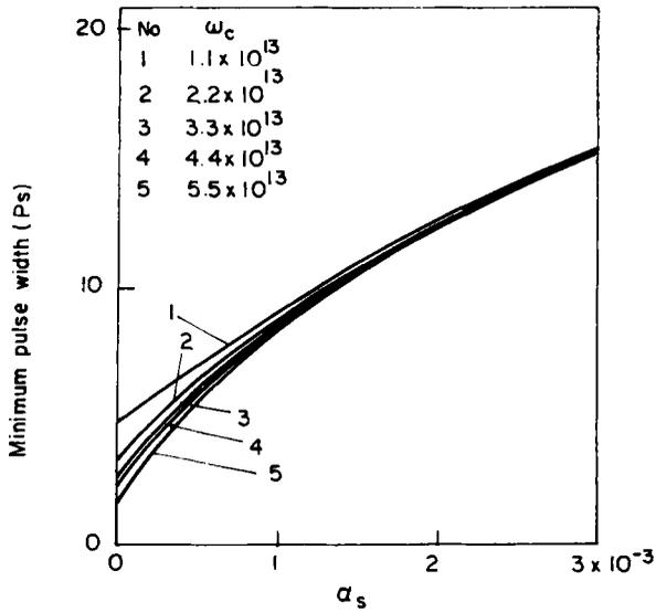
Figure 2. Variation of minimum pulsedwidth with harmonic conversion efficiency for constant intracavity bandwidth.
