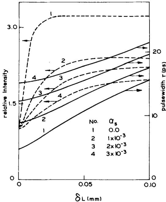
Figure 1. Pulsewidth and peak intensity of pulse as functions of cavity mismatch for different conversion efficiencies.
