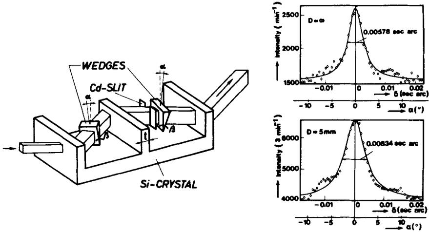
Figure 3. Experimental arrangement for the observation of the narrow central peak of multiple Laue rocking curves (left) and a typical slit diffraction pattern (Rauch *et al* 1983).
