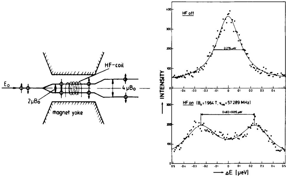
Figure 6. Verification of the coherent energy shift of a neutron magnetic resonance system (Alefeld *et al* 1981).
