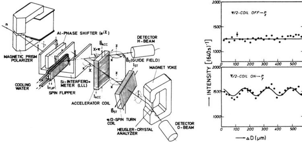
**Figure 5.** Experimental arrangement and results of the static spin superposition experiment (Summhammer *et al* 1982).
