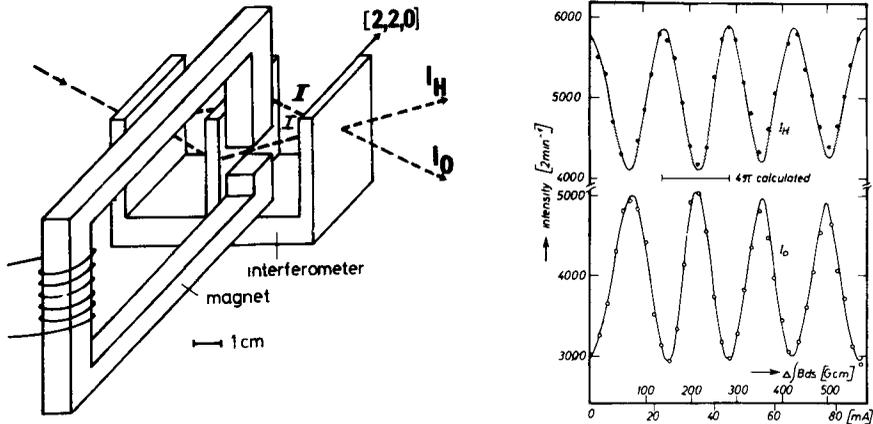
Figure 4. First observation of the  $4\pi$ -symmetry of a spinor wave function (Rauch *et al* 1975).
