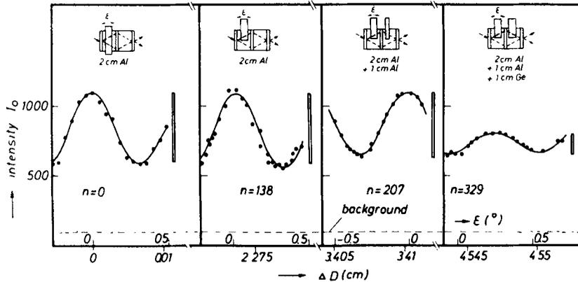
**Figure 2.** High order interferences and the reduction of the contrast due to the wavelength spread of the beam (Rauch 1979).
