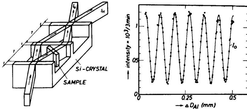
**Figure 1.** Sketch of a perfect crystal neutron interferometer (left) and a typical interference pattern (right).
