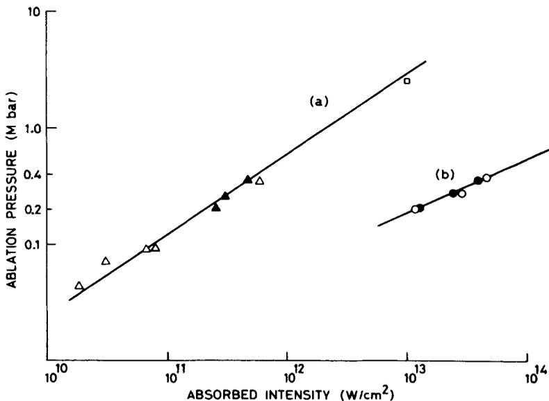
**Figure 4.** Scaling of ablation pressure with absorbed laser intensity **a.** for a focal spot of diameter of  $500\ \mu\text{m}$  and **b.** for a focal spot diameter of  $30\ \mu\text{m}$ .  $\blacktriangle$ ,  $\bullet$ —Results of double foil experiments.  $\Delta$ ,  $\circ$ —Results of single foil experiments.  $\square$ —A data point corresponding to NRL experiments.
