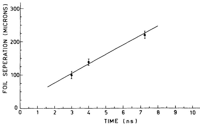
**Figure 3.** Impact time data to determine target foil velocity. Foil separation plotted against impact time.
