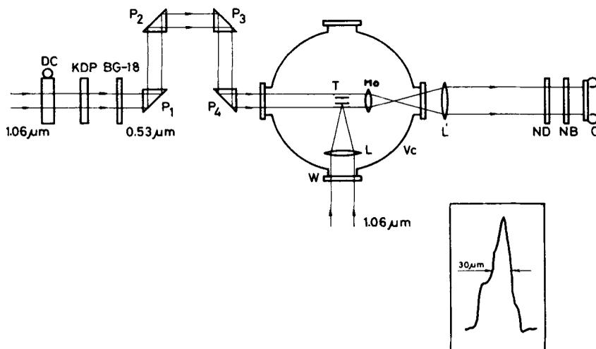
**Figure 1.** Experimental set up. T-Target foils, L-Focussing lens, W-Window, Vc-Vacuum chamber, Mo-Microscope objective, L'-imaging lens, ND, NB-Filters, C-Camera, DC-Saturable absorber cell, KDP-KDP crystal for second harmonic generation, BG-18-Green filter to cut off residual  $1.06 \mu\text{m}$  beam,  $P_1$ ,  $P_2$ ,  $P_3$ ,  $P_4$ -Folding prisms for optical delay.
