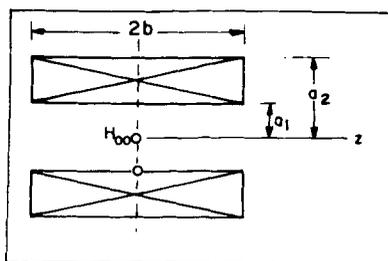
Figure 2. Coordinate system of coil configuration.
