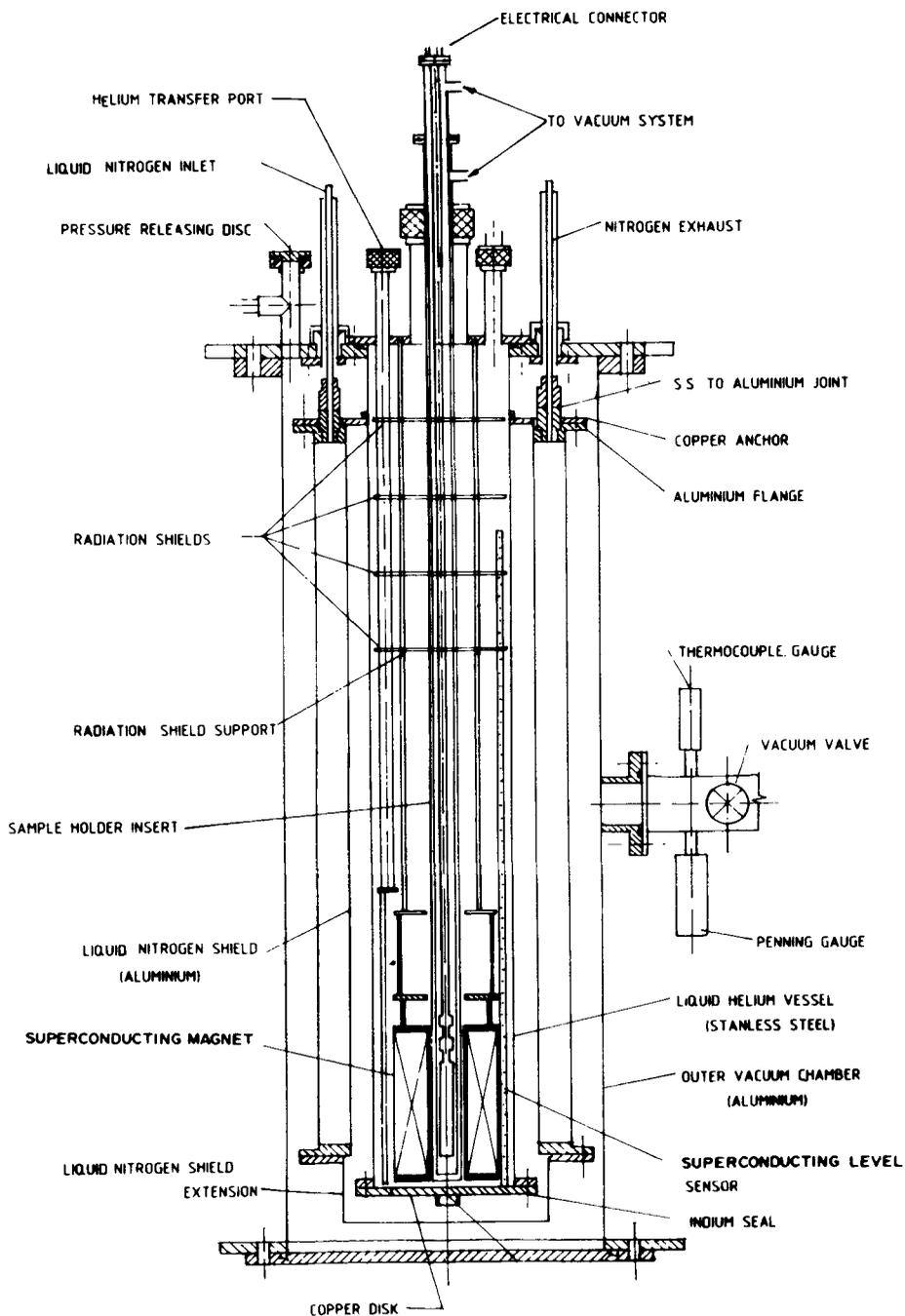
Figure 1. Schematic diagram of the complete magnetoresistance set-up.
