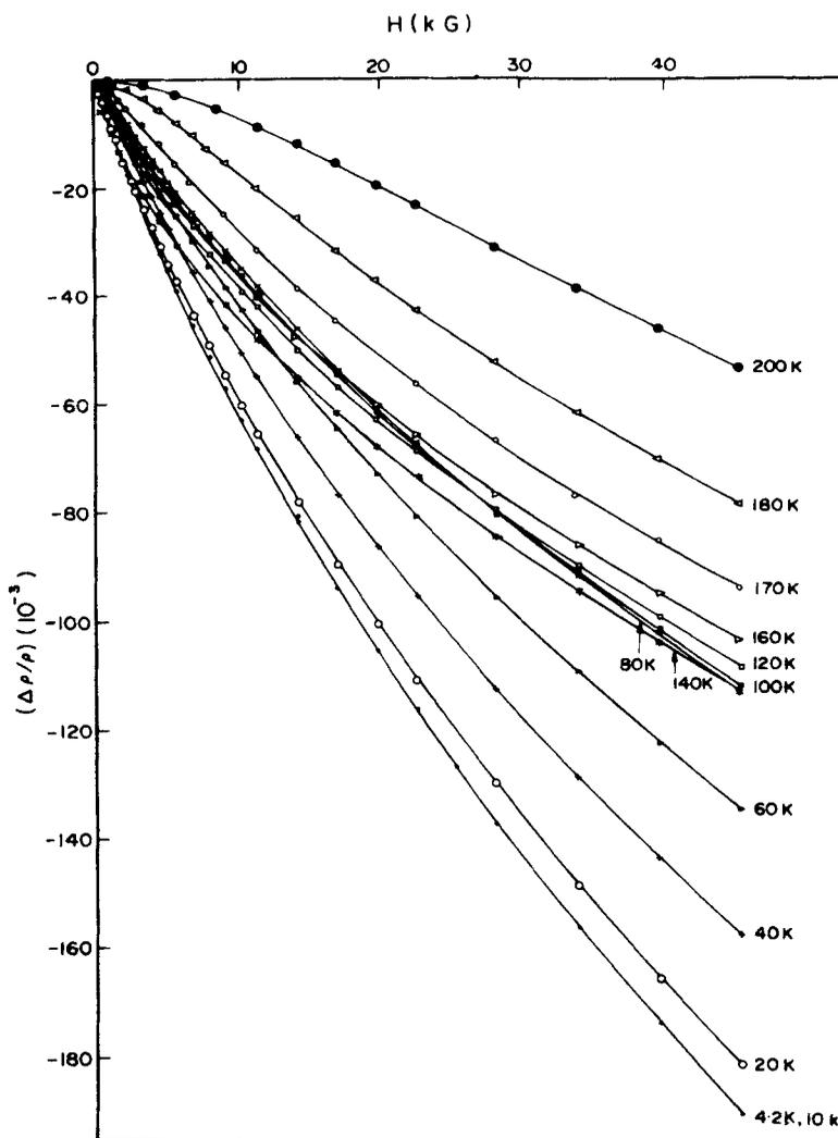
**Figure 8.** Variation of magnetoresistance with field at various temperatures in the range 4.2–200 K, as measured in the present set-up.
