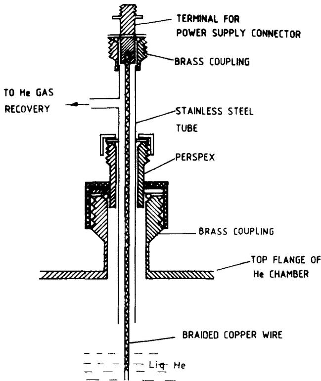
**Figure 4.** Schematic diagram of the vapour cooled current leads for the superconducting magnet.
