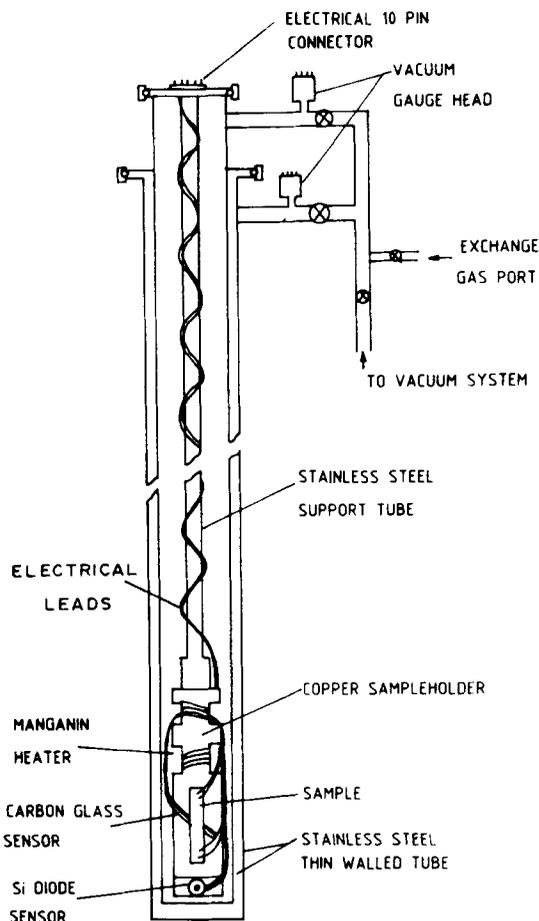
**Figure 5.** Sample holder insert assembly for magnetoresistance study.
