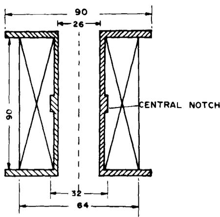
Figure 3. Notched coil-form used in the construction of the superconducting magnet for improved homogeneity (all dimensions in mm).
