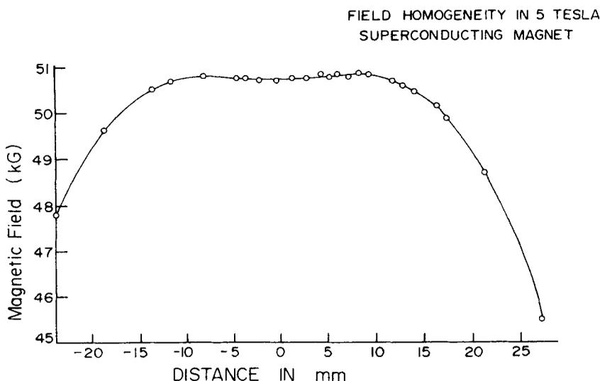
**Figure 7.** Magnetic field profile along the axis of the superconducting magnet solenoid. Note that the field has a homogeneity of about 0.2% over a length of 20 mm around the centre.
