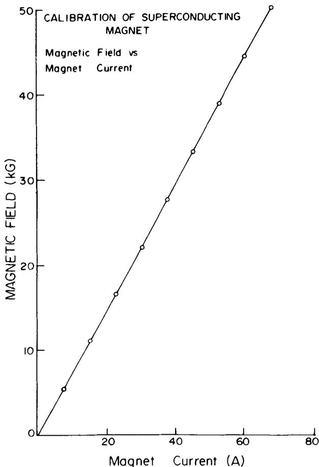
Figure 6. Field calibration of the superconducting magnet against magnet current.
