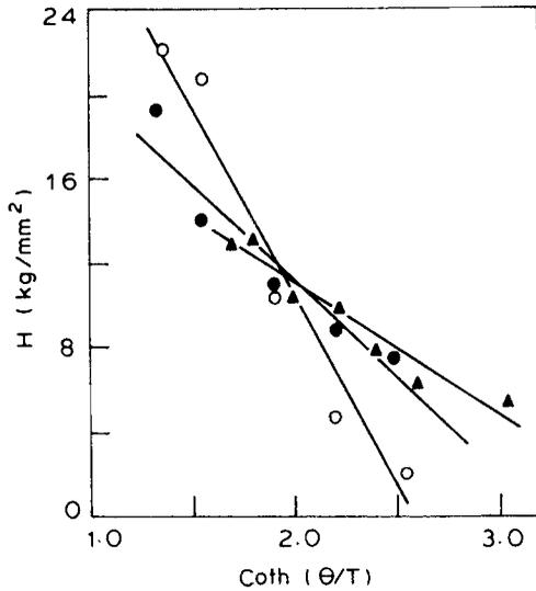
Figure 4. Plot of hardness ( $H$ ) against  $\cot h(\theta/T)$  (symbols as in figure 2).
