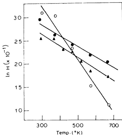
Figure 2. Plot of  $\log H$  against temperature ( $T$ ):  $\circ$ —NaCl present data,  $\bullet$ —Boyarskaya (1972),  $\blacktriangle$ —KCl.
