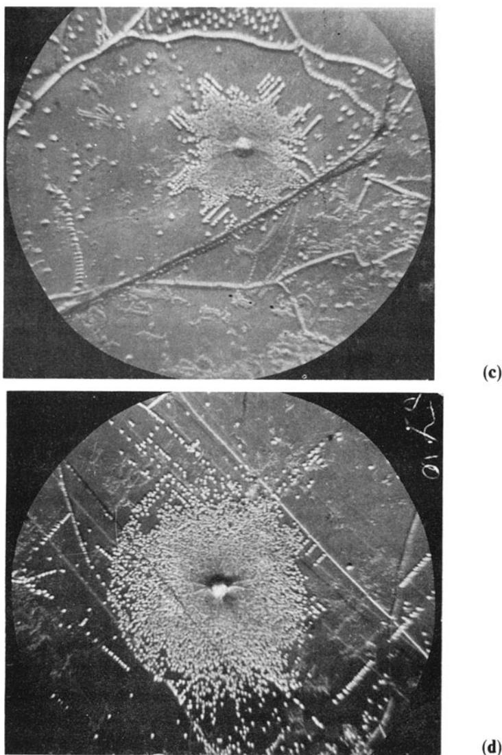
**Figure 1.** ( $\times 100$ ) IDR patterns for NaCl at various temperatures **a.** 30°C, **b.** 200°C, **c.** 300°C, **d.** 400°C. The arms of the rosette are in the  $\langle 110 \rangle$  directions.
