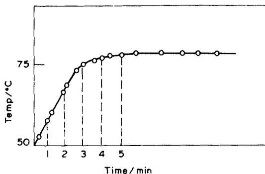
**Figure 4.** Temperature rise for a sharp power increment to the cell. It is noted that the steady state is achieved within 5 min.
