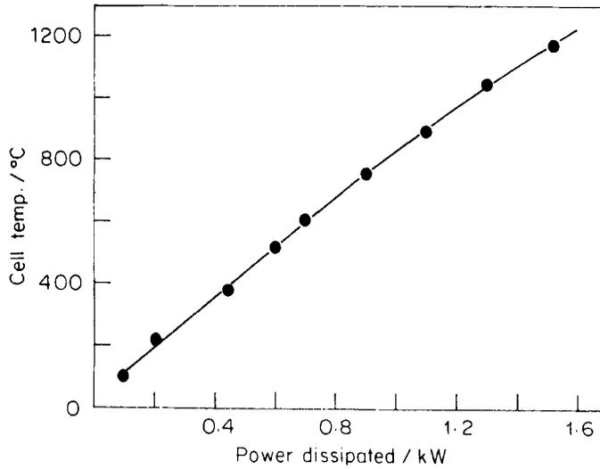
**Figure 9.** Power input vs temperature data. The plot is observed to be linear up to 600°C, beyond which a decrease in slope can be seen.
