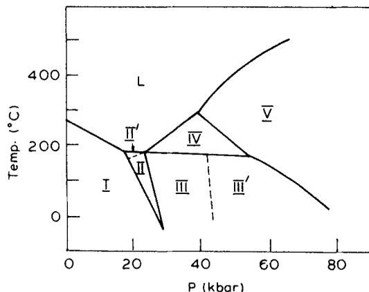
**Figure 6.** Bismuth phase diagram. At least 8 polymorphic phases can be visualized under hp-ht. Up to 15 kbar,  $T_m$  decreases with pressure and beyond it up to 26 kbar, it is almost constant. Beyond 26 kbar  $\partial T_m/\partial P$  is positive, characteristic of any normal metal.
