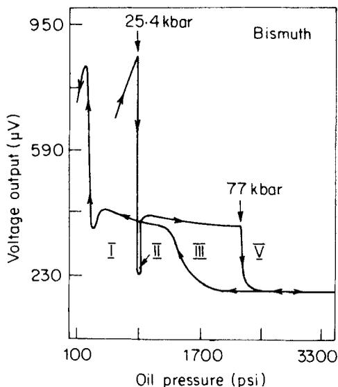
**Figure 7.** Electrical resistivity data obtained on Bi at room temperature. 25.4 kbar (I-II), 27 kbar (II-III), and 77 kbar (III-IV) can easily be identified. Hysteresis is remarkable.
