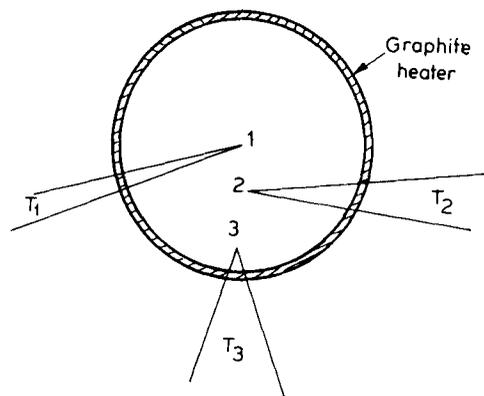
**Figure 3.** Three thermocouples distributed inside the graphite furnace to check the temperature gradient inside the experimental region. We find that the difference in temperature between the thermocouples at the centre and at the extreme end is less than  $5^{\circ}\text{C}$  in the steady state.
