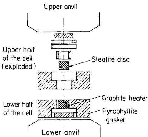
**Figure 2.** High pressure-high temperature cell assembly. The assembly, as can be seen consists of two symmetrical parts where pyrophyllite has been used in split gasket configuration. Current path is established through anvil → graphite ring → disc → ring → anvil. Pyrophyllite is used to contain the pressure. Silver chloride is used as pressure transmitting medium.
