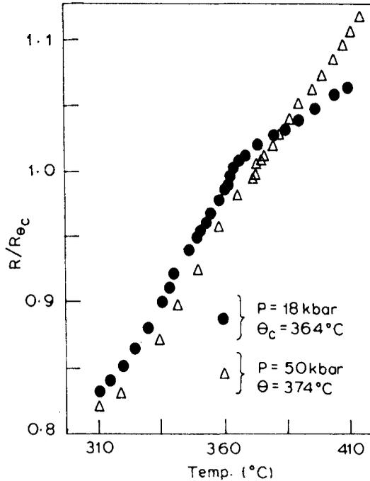
**Figure 12.** High pressure-high temperature electrical resistivity data on Ni as a test problem.  $T_c$  increases with pressure. Also the temperature coefficient of electrical resistivity increases with pressure for temperatures beyond  $T_c$ .
