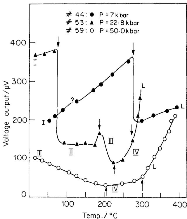
**Figure 11.** Electrical resistivity data on Bi under high pressure and high temperature. (●) indicate that at 7 kbar, Bi melts at 270°C. At 22.8 kbar, (▲) indicate I  $\xrightarrow{70^\circ\text{C}}$  II  $\xrightarrow{170^\circ\text{C}}$  III  $\xrightarrow{220^\circ\text{C}}$  IV  $\xrightarrow{270^\circ\text{C}}$  L. At 50 kbar, (○) indicate III  $\xrightarrow{200^\circ\text{C}}$  IV  $\xrightarrow{300^\circ\text{C}}$  L.
