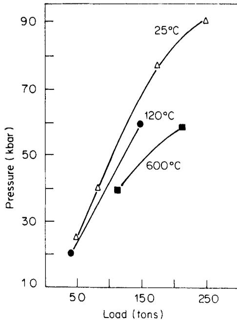
**Figure 10.** Press calibration curve. It is seen that the slope of the load vs pressure curve decreases slowly with temperature. At the moment, it is incomplete.
