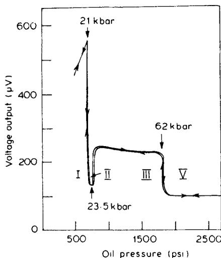
**Figure 8.** Electrical resistivity data of Bi under high pressure and at a temperature of 120°C. The return cycle indicate that hysteresis is very small at this temperature.
