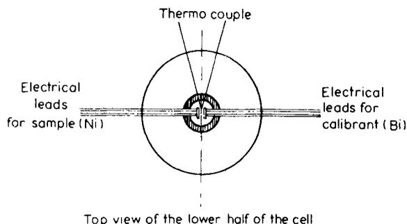
**Figure 5.** Arrangement showing the placement of the sample (with 4-probes), calibrant (with 4-probes) and the thermocouple to monitor the temperature very near the sample and the calibrant.
