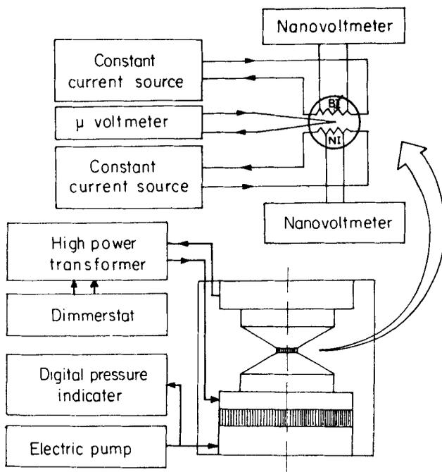
**Figure 1.** The experimental set-up. Electrically driven hydraulic pump is used to generate the load in the hydraulic press and the oil pressure read by a digital pressure indicator. A high power transformer controlled by the dimmerstat is used to power the graphite furnace, used as internal heater to the sample under investigation.
