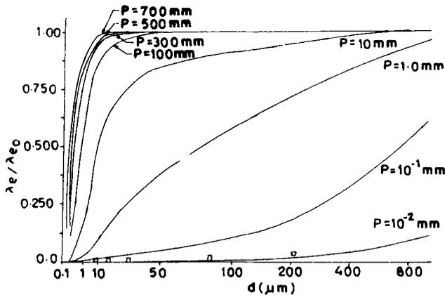
Figure 2. Variation of  $\lambda_e$  with pore diameter  $d$  through (17) at different interstitial air pressure. The symbol ( $\square$ ) represents the experimental value of  $\lambda_e$  of glass beads of different sizes at the interstitial air pressure of  $10^{-2}$  mm of Hg. (Wechsler *et al* 1972).
