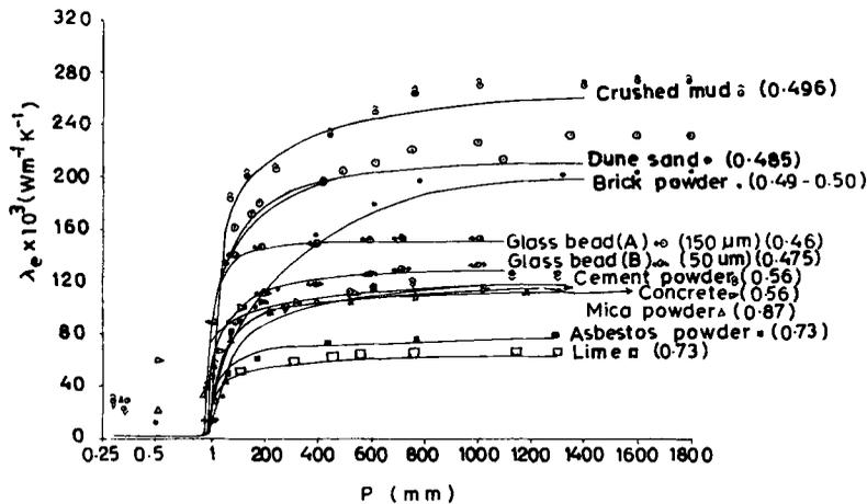
**Figure 1.** Effective thermal conductivity of loose building-materials and glass beads at varying interstitial air pressures. The continuous lines represent the calculated values of  $\lambda_e$  through (17) while the symbols represent the experimental values (Pande *et al* 1984; Wechsler and Glaser 1964).
