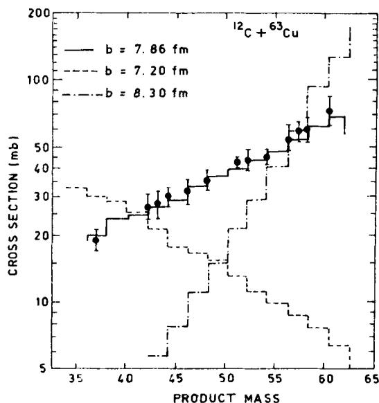
Figure 3. Impact parameter dependence of the mass yield distribution of  $^{12}\text{C} + ^{63}\text{Cu}$  reaction.
