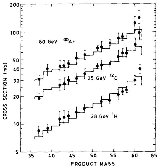
**Figure 1.** Calculated limiting mass yield distribution for fragmentation of Cu target. The histograms are for 28 GeV p, 25 GeV  $^{12}\text{C}$  and 80 GeV  $^{40}\text{Ar}$  projectiles. Data (solid dot) taken from Cumming *et al* (1978).
