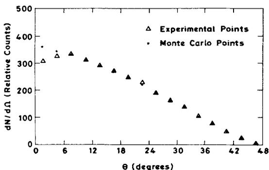
Figure 1. Calculated (Monte-Carlo) and experimental angular distributions of LRA s emitted in thermal-neutron induced fission.
