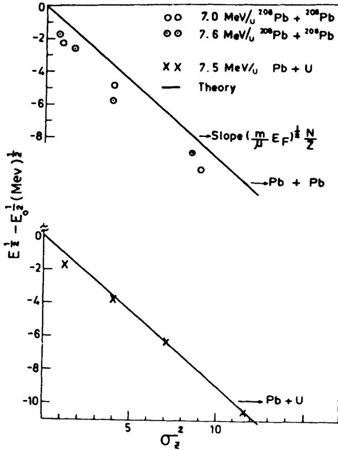
Figure 5. Plots of  $E^{1/2}$  versus  $\sigma_z^2$  for  $7.0 \text{ MeV/u Pb} + \text{Pb}$ ,  $7.6 \text{ MeV/u Pb} + \text{Pb}$  and  $7.5 \text{ MeV/u Pb} + \text{U}$ .
