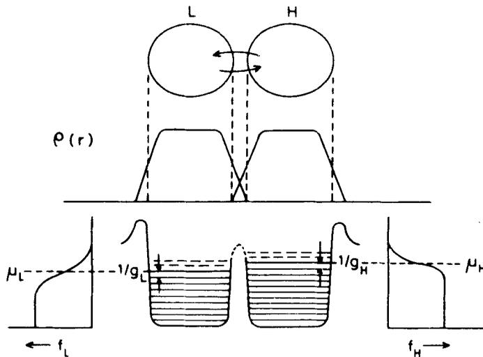
**Figure 1.** Schematic diagram illustrating the nucleon exchange mechanism between the fragments  $L$  and  $H$ .  $\rho_{L/H}(r)$  represents the diffuse densities,  $g_{L/H}$  are the single particle level densities,  $f_{L/H}$  are the Fermi-Dirac occupation probabilities and  $\mu_{L/H}$  are the chemical potentials of the fragments  $L$  and  $H$  respectively.
