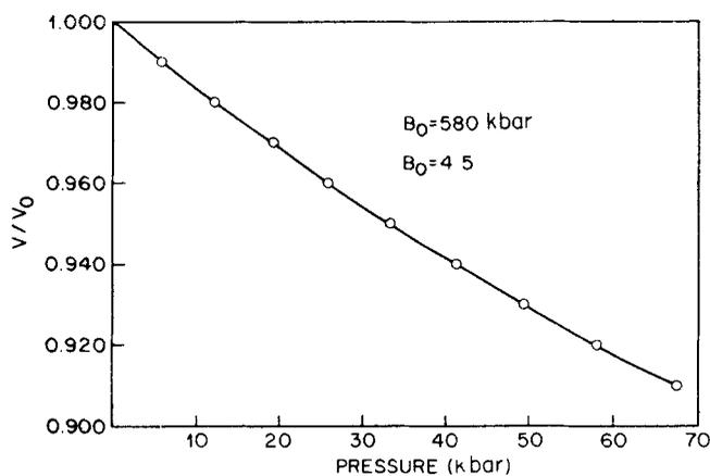
**Figure 3.** Pressure-volume relationship for InAs obtained from the Birch-equation of state.
