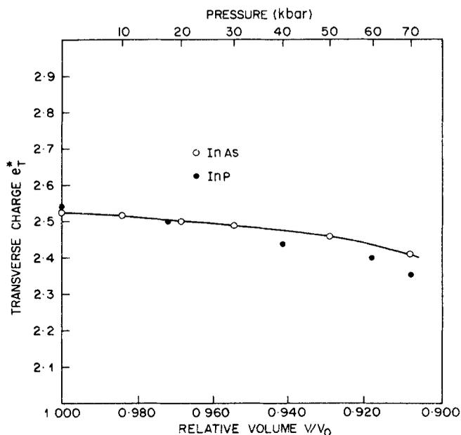
**Figure 4.** Born's transverse charge plotted against relative volume. The pressure scale is on top. The filled circles are the data points for InP.
