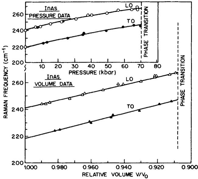
**Figure 2.** A plot of the LO-TO phonon frequency against pressure (top) and against relative volume (bottom). The dotted line indicates the disappearance of the phonons and the phase transition.
