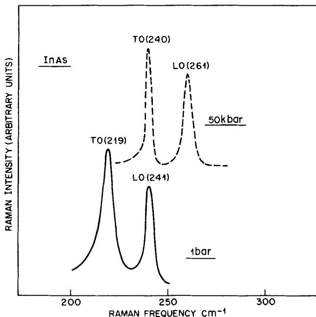
Figure 1. The LO-TO phonons in InAs at ambient pressure and at a pressure of 50 kbar.
