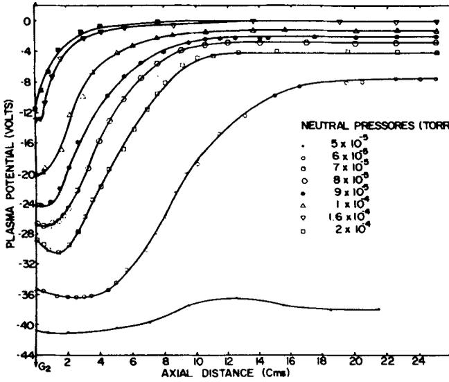
Figure 13. Axial plasma potential profiles in the target chamber at different neutral pressures, keeping the relative bias voltage and grid bias voltages constant.
