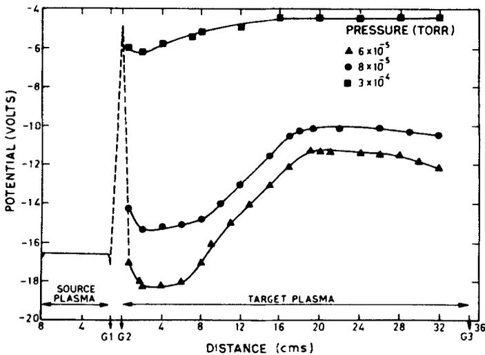
Figure 5. Axial potential profiles in the target chamber at different pressures and a fixed relative bias. Profile A (■) corresponds to the shallow potential structure and profile C (Δ) corresponds to the double-layer potential profile.
