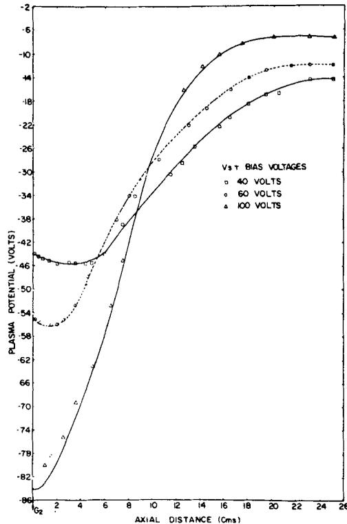
**Figure 10.** Axial plasma potential profiles in the target chamber, at different relative bias voltages varied from 40–100 V.
