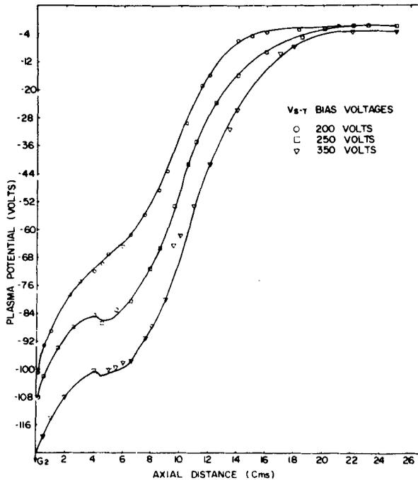
**Figure 11.** Axial plasma potential profiles in the target chamber, at different relative bias voltages varied from 200–350 volts. Note the presence of a knee-like structure and a clear potential dip after the sheath-like structure. This closely resembles the multiple double layers.
