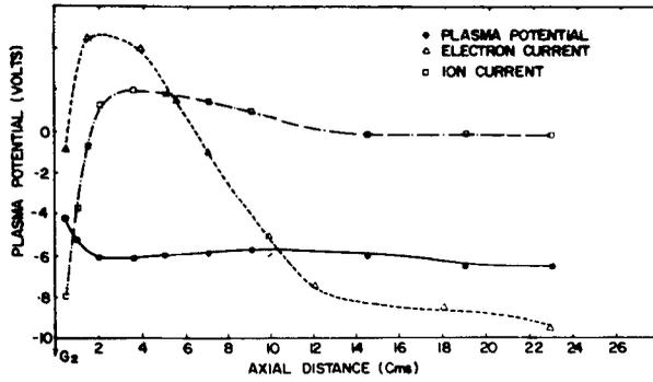
Figure 15. Plots of plasma potential, electron current and ion current in the target chamber, in the absence of a double layer. Electron currents are in mA, and ion currents are in  $\mu A$ .
