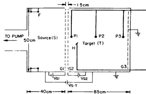
**Figure 1.** Schematic of the double plasma machine. Drifting electrons are produced by biasing the source chamber negative with respect to the target chamber. F—Filaments,  $P_1$ ,  $P_2$ ,  $P_3$ —collecting Langmuir probes, H—emissive probe. Grid G1 is biased 0 V with respect to the source, potential of grid G2 is varied from 0–10 V with respect to the target and the end grid G3 is grounded.
