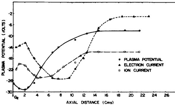
Figure 17. Plot of plasma potential (thick line), electron current (dashed lines) and ion current (dot and dashed lines), in the target chamber in the presence of a strong double layer. The electron and ion currents are in mA and  $\mu A$  respectively.
