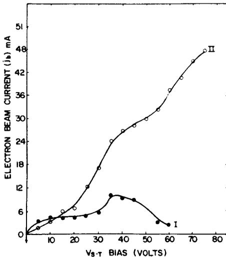
**Figure 18.** Plot of the beam electron current in the two configurations I and II vs  $V_{S-T}$ . The current was monitored at a distance of 2 cm from the grid G2 in the target region, with a Langmuir probe biased to collect energetic electrons.
