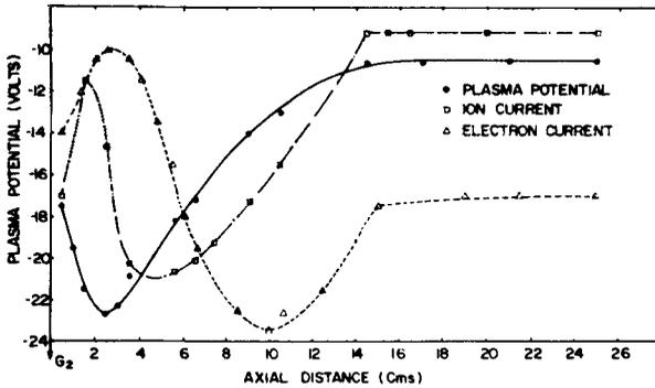
Figure 16. Plot of the plasma potential (thick line), electron current (dashed lines), ion current (dot and dashed lines), in the target chamber when a weak double layer was formed. The electron and ion currents are in mA and  $\mu A$  respectively.
