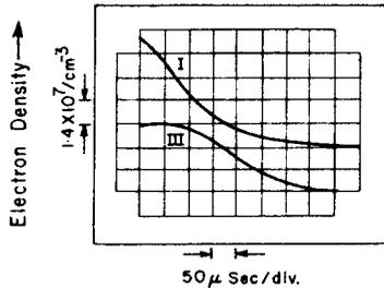
**Figure 3.** Oscilloscope trace of time profile of the saturation electron currents obtained by collecting Langmuir probe  $P_1$  and  $P_3$ . Figure shows that the arrival of the plasma blob at  $P_3$  is delayed by  $\approx 30 \mu\text{sec}$  with respect to the same at  $P_1$ .
