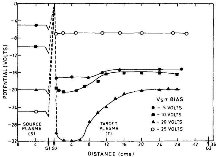
**Figure 7.** Axial potential profiles in the target chamber at different relative bias voltages, keeping the pressure constant. Profile B(0) corresponds to the shallow potential structure, at a large relative bias.
