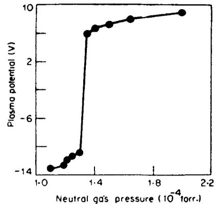
**Figure 4.** The plasma potential near G2 is plotted for various neutral gas pressures. The device control settings are  $G1 = 0 \text{ V}$  and  $G2 = 10 \text{ V}$ ,  $G3$  is grounded and  $V_{S-T} = -8.3 \text{ V}$ . Note the sharp transition in the plasma potential between  $1.3$  and  $1.35 \times 10^{-4} \text{ torr}$ .
