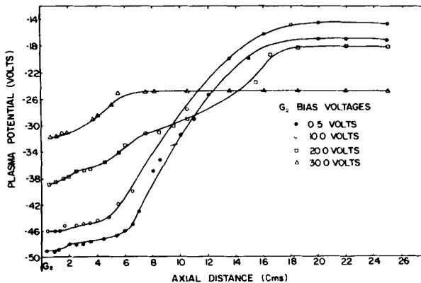
**Figure 12.** Axial plasma potential profiles in the target chamber at different G2 bias voltages keeping the relative bias voltages and neutral pressure constant.
