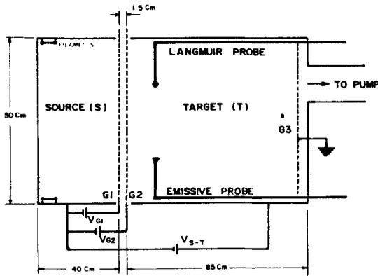
**Figure 8.** Configuration II, modified to obtain strong double layers. Grids G1 and G2 have been biased with respect to source, and the pumping unit is on the target region with gas feed in source region. Drifting electrons are injected from the source into the target chamber by the relative bias. G1 and G2 are normally biased to 0 V.
