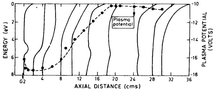
**Figure 6.** Electron energy distribution functions at various space points corresponding to profile C of figure 5. The potential profile is represented by dashed line. Drifting electron distribution is present on the low potential side and accelerated component which thermalises in a distance of about 10 cm is present on the high potential side.
