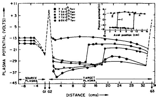
**Figure 2.** The axial plasma potential profiles in the target chamber at various indicated pressures, obtained by the emissive probe. The inset is a typical potential variation at the critical pressure. Profile A corresponds to when the emissive probe is moved away from the grid G2, and profile B, when the emissive probe is moved towards grid G2. The dashed line (branch II of the profile B) shows that occasionally the entire plasma potential is at high state.
