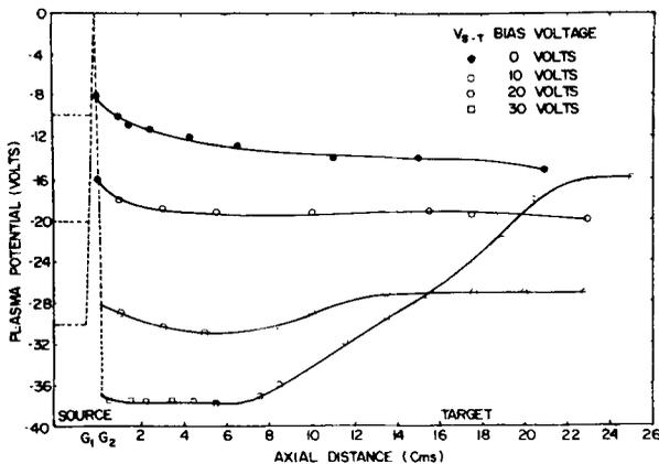
**Figure 9.** Axial plasma potential profile in the target chamber, at different relative bias voltages varied from 0–30 V.
