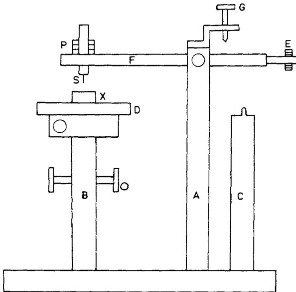
Figure 1(b). Line diagram of the indenter.
