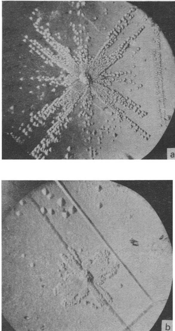
**Figure 3.** ( $\times 300$ ) Indentation dislocation rosette pattern on (a). Pure NaCl (b). Sr-doped NaCl.
