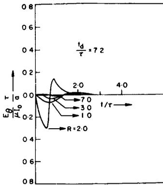
Figure 13. Time variation of the azimuthal electric field at different radius.
