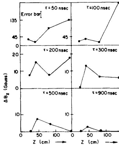
Figure 8. Spatial behaviour of magnetic perturbation at different intervals of time. The horizontal axis represents the distances marked from the cusp plane. The mirror centre is at 70 cm, and grid at 155 cm.
