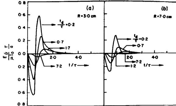
Figure 12. Azimuthal electric field as function of time for different conductivities outside the beam cross-section.
