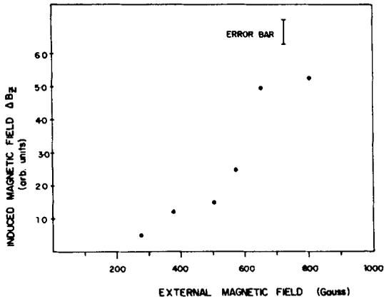
Figure 19. Dependence of the beam induced axial magnetic field  $\Delta B_z$  on the external magnetic field  $B_0$ .
