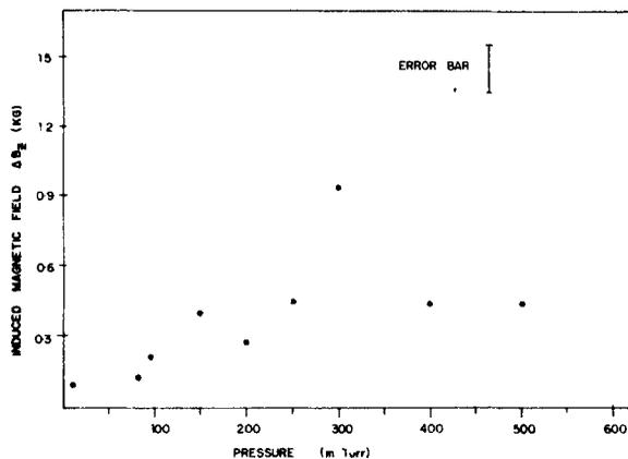
Figure 18. Variation of the induced axial magnetic field with neutral gas pressure.
