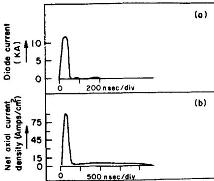
**Figure 4.** (a) A typical diode current output (b) Net axial current density as function of time obtained at 20 mm radial position.
