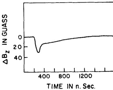
Figure 7. A diamagnetic loop output showing the magnetic perturbation at the mirror centre as a function of time.
