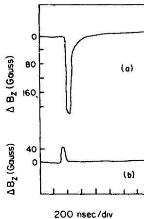
Figure 3. The diamagnetic loop output measured (a) at the inner side of the grid with loop B, (b) at a point outside the grid with loop A.
