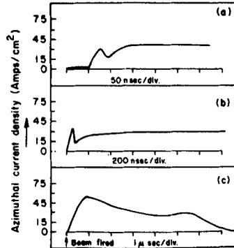
**Figure 5.** Time evolution of the net azimuthal current.
