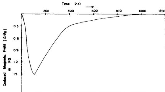
Figure 16. Time evolution of the diamagnetic loop when rotating electron beam is injected into neutral gas.
