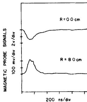
Figure 17. Magnetic probe output on and off axis.
