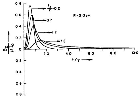
Figure 14. Dependence of the induced axial magnetic field at the axis on plasma conductivity.
