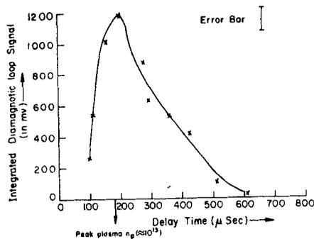
Figure 9. Dependence of the peak diamagnetic loop signal on the time delay between the beam generator and the plasma gun firing.
