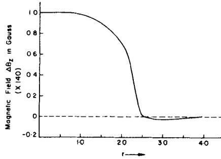
Figure 6. Radial profile of the beam induced axial magnetic field.
