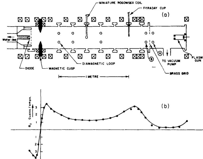
Figure 1. Schematic of the experimental set-up and magnetic field profile.
