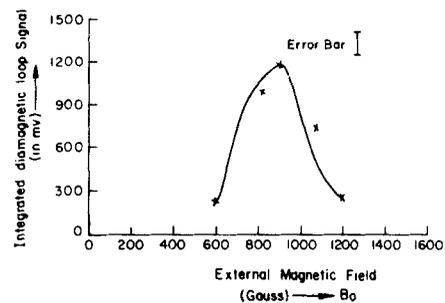
Figure 10. Dependence of the peak diamagnetic loop on the external magnetic field. Horizontal axis represents the field at the mirror point.
