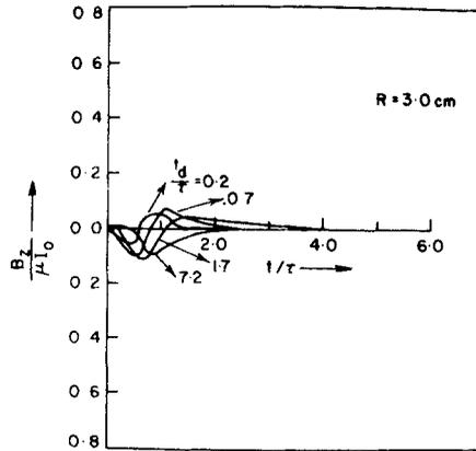
Figure 15. Induced axial magnetic field's time profile at 30 mm radius.
