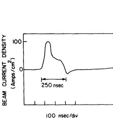
Figure 2. Electron beam current density, measured with an energy selective electron probe at the mirror centre.
