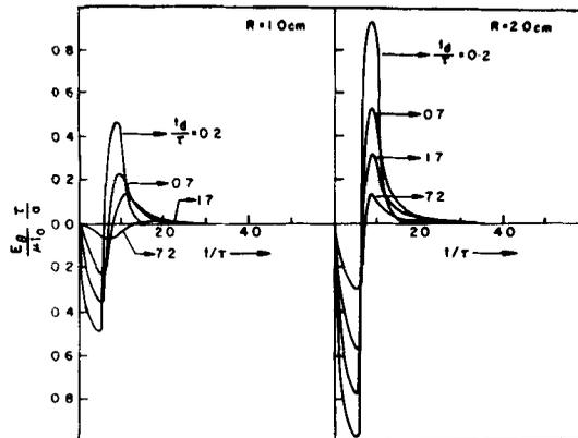
Figure 11. Azimuthal electric field as function of time for different conductivities within the beam radius. Here  $\tau$  is the beam pulse duration,  $\tau_d = 4\pi\sigma^* a^2/c^2$ ,  $a$  is the beam radius,  $I_0$  is the peak beam current per unit length.
