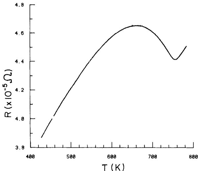
Figure 6. Electrical resistance of a sample of 16 at. % Mn in Cr alloy as a function of absolute temperature. The  $R$  vs.  $T$  curve contains about 2500 data points.
