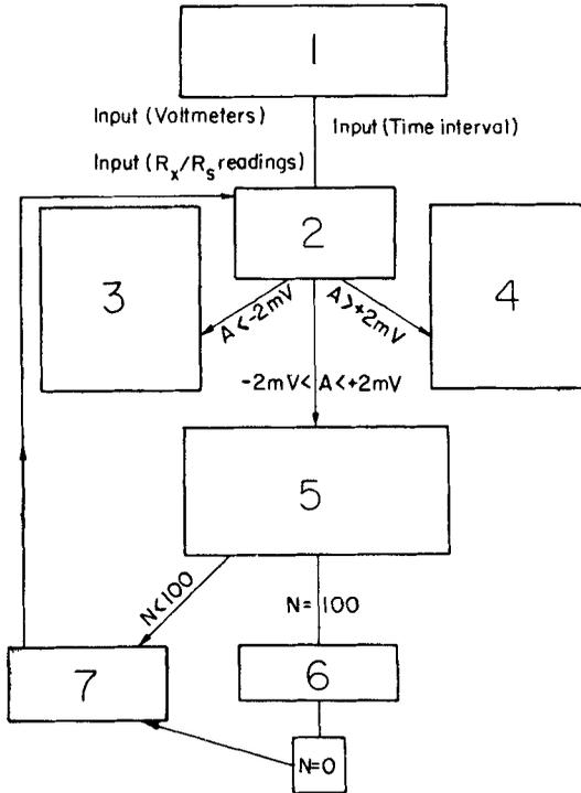
**Figure 3.** Program of the system. 1. Initiate all ports, variables, time, and IEEE-488 interface board, 2. Read the output of the bridge galvanometer A, 3. Decrease the  $R_x/R_s$  dial readings, 4. Increase the  $R_x/R_s$  dial readings, 5. Read the voltmeters in use, store readings, and corresponding  $R_x/R_s$  values, 6. Store the block of 100 data sets, 7. Delay for the determined time interval.
