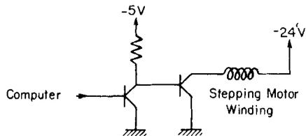
**Figure 4.** Darlington pair transistor and winding configuration of the stepping motor.
