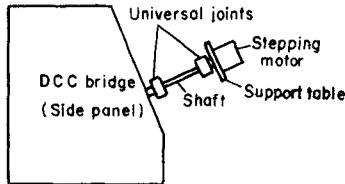
Figure 1. Side view of the direct current comparator resistance bridge and its accessories.
