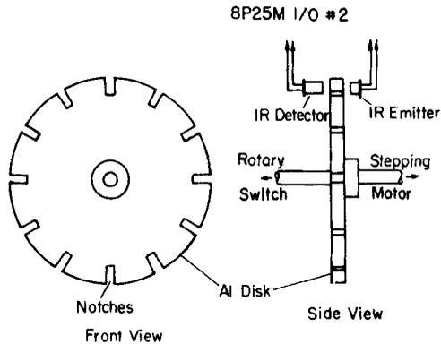
Figure 5. IR emitter and detector positions with the notched disk.
