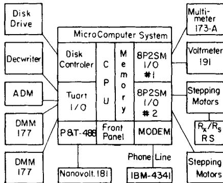
Figure 2. Block diagram of the system.
