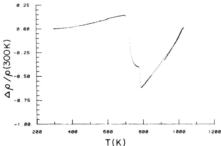
**Figure 7.** Relative change of the electrical resistivity of glassy metal  $\text{Fe}_{83}\text{B}_{14}\text{Si}_3$  (with 21 ppm of N) undergoing crystallization as a function of the absolute temperature.  $\Delta\rho = \rho(T) - \rho(300\text{K})$ , where  $\rho(T)$  is the electrical resistivity at the absolute temperature  $T$ . Heating rate  $\approx (6-8)\text{K/min}$ . Data taken every 2 K.
