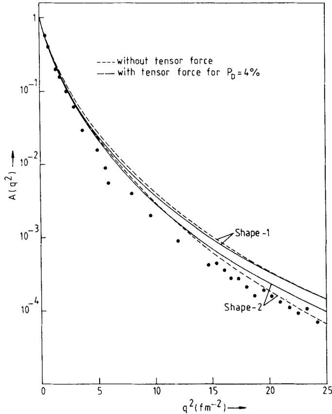
**Figure 3.** Deuteron form factor  $A(q^2)$  for potential sets without and with tensor force ( $P_D = 4\%$ ). Experimental points are from Elias *et al* (1969).
