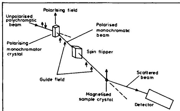
Figure 3. Schematic diagram of a polarised beam diffractometer.
