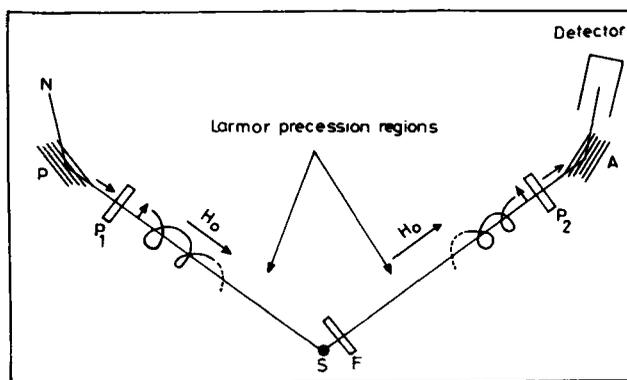
**Figure 7.** Schematic diagram of a focussed spin-echo spectrometer.  $N$ : Unpolarised incident beams;  $P$ ,  $A$ : polariser and analyser,  $P_1$ ,  $P_2$ :  $\pi/2$  spin turn coils.  $F$ :  $\pi$  spin turn coil.  $S$ : Sample.  $H_0$ : guide field (shown solenoidal here).
