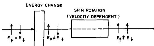
Figure 5. Principle of dynamical polarisation.
