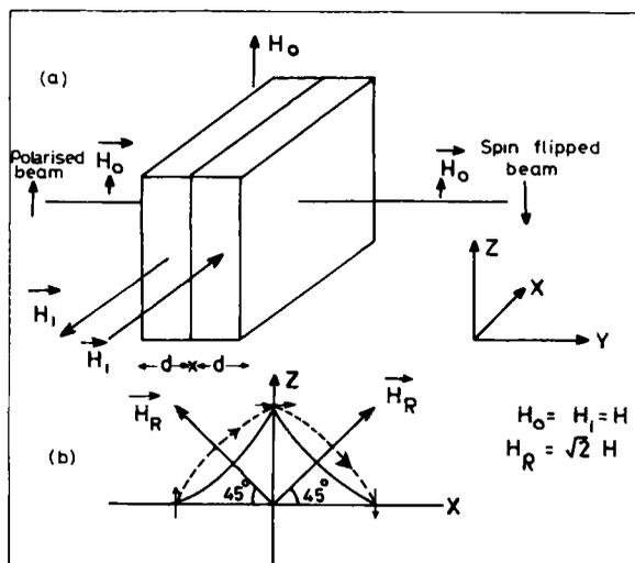
Figure 1. (a) Mezei flipper coils (b) the rotation of the neutron spins in the two coils.
