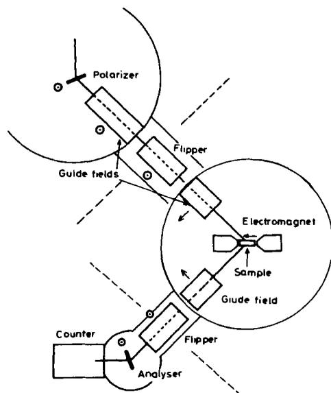
Figure 6. Schematic diagram of a polarisation analysis spectrometer.
