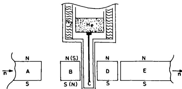
Figure 2. Non-adiabatic spin flipper system that uses an isolating sheet of superconducting niobium (see text).
