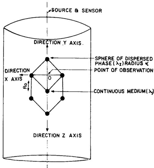
**Figure 1.** Cylindrical sample container containing the material (two-phase system) with source and sensor.
