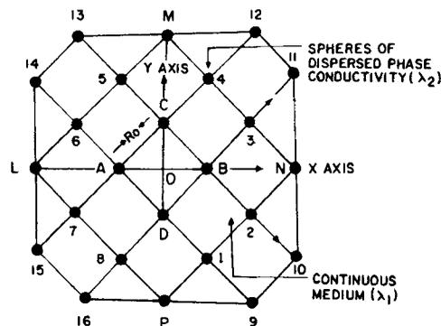
**Figure 2.** A lattice plane of dispersed spheres around the sensor in X-Y plane.
