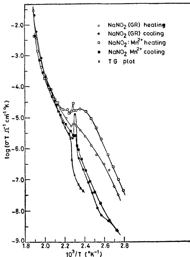
Figure 1. The temperature dependence of electrical conductivity  $\sigma$  for the undoped and  $\text{Mn}^{2+}$ -doped  $\text{NaNO}_2$  single crystals in heating and cooling runs.
