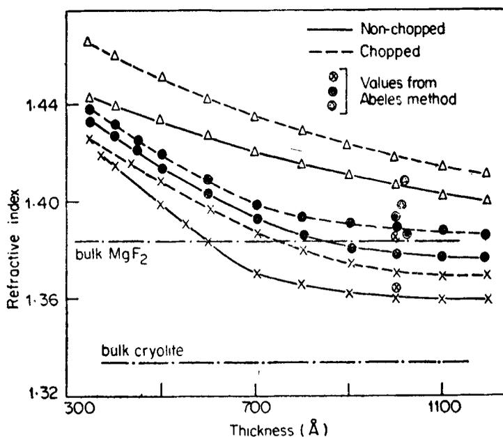
Figure 3. Average initial refractive index versus thickness as measured by ellipsometer at  $\lambda = 6328 \text{ \AA}$ , X cryolite,  $\Delta$  MgF<sub>2</sub>, ● mixed cryolite-MgF<sub>2</sub>. Temperature of substrate: Room temperature (27°C).
