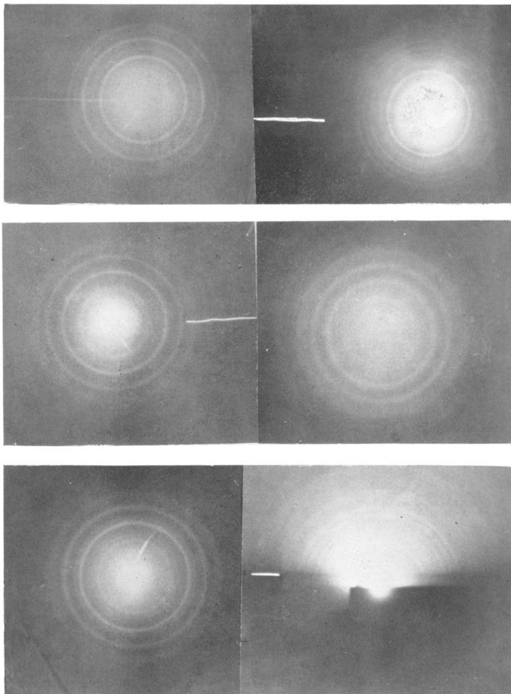
**Figure 5.** Electron diffraction pattern. a1, b1, c1 Non-chopped cryolite,  $\text{MgF}_2$  and mixed cryolite- $\text{MgF}_2$  respectively. a2, b2, c2 chopped cryolite,  $\text{MgF}_2$  and mixed cryolite- $\text{MgF}_2$  respectively.
