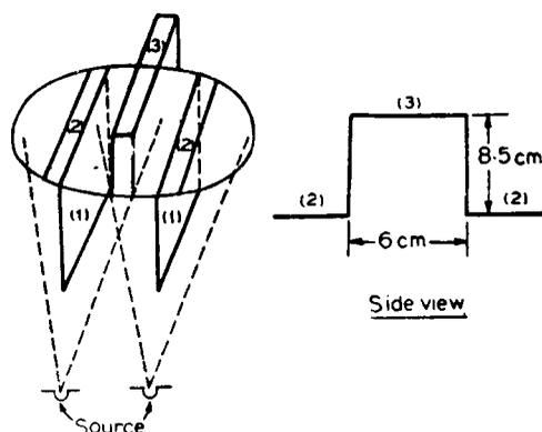
Figure 1. Schematic diagram of the shadowing arrangement for deposition of single and mixed films. (1) Projection for shadowing, (2) Side slots, (3) Central slot.
