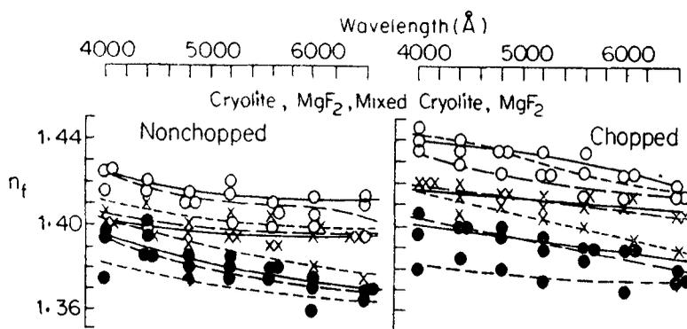
Figure 2. Wavelength dependence of the average, initial refractive index. ● cryolite, ○ MgF<sub>2</sub>, X Mixed cryolite-MgF<sub>2</sub>, Thickness: — ~ 700 Å, - - - ~ 900 Å, - · - · ~ 1100 Å Temperature of substrate: Room temperature (27°C).
