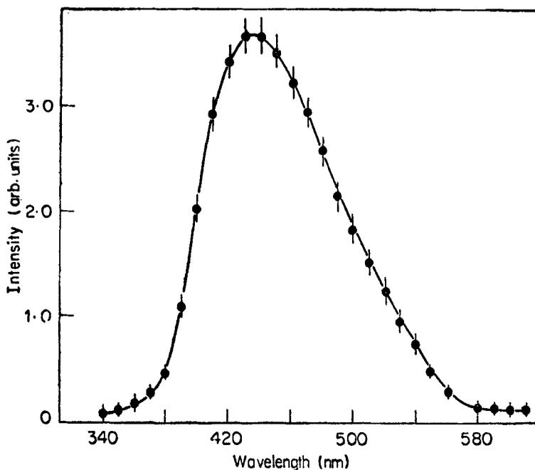
Figure 7. ML spectra of irradiated KCl crystals.
