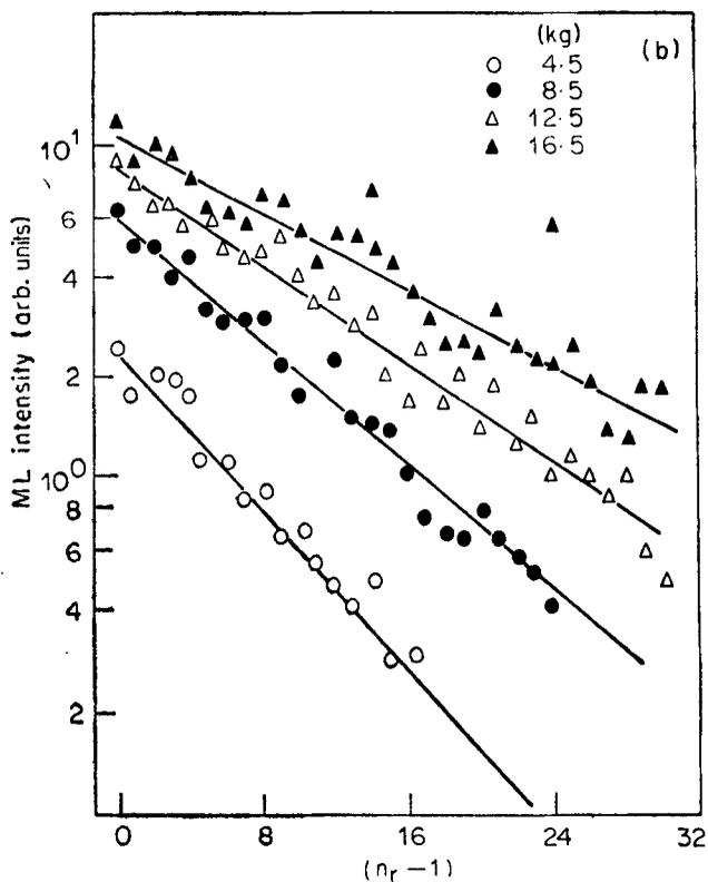
Figure 3. Plot of log ML intensity vs a.  $(n_p - 1)$  b.  $(n_r - 1)$  in  $\gamma$  irradiated KCl crystals for different values of uniaxial pressure.
