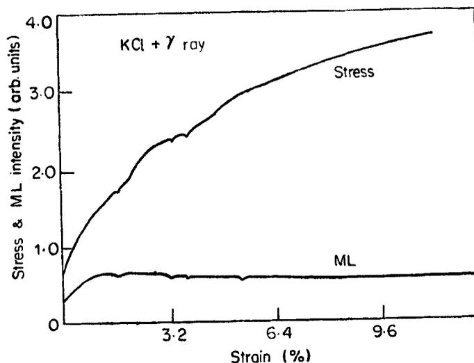
Figure 1. Mechanoluminescence vs compression and the force vs compression curves for  $\gamma$  irradiated KCl crystal.
