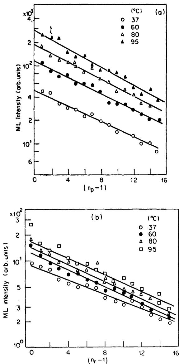
Figure 4. Plot of log ML intensity vs a.  $(n_p - 1)$  b.  $(n_r - 1)$  in  $\gamma$  irradiated KCl crystals for different values of temperature.
