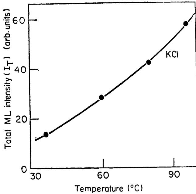
Figure 5. Effect of temperature on the total ML intensity  $I_T$  of  $\gamma$  irradiated KCl crystals.
