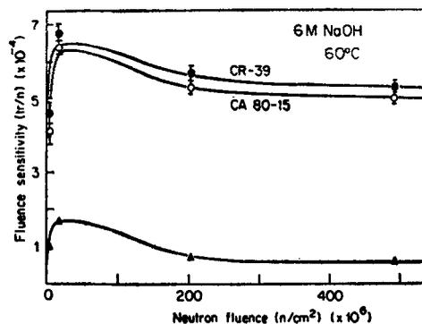
Figure 3. Variation of sensitivity with neutron fluence.
