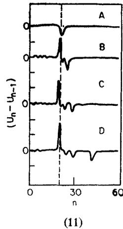
Figures 9-11. 9. Collision of two solitons at a vacancy at the place of 30th atom in the chain of 60 atoms. 10, 11. Propagation of soliton in a medium with density discontinuity. 10. Propagation of soliton from a rarer to denser medium 11. Propagation from a denser to rarer medium. X axis 1 cm=10 atoms, Y axis=1 Å
