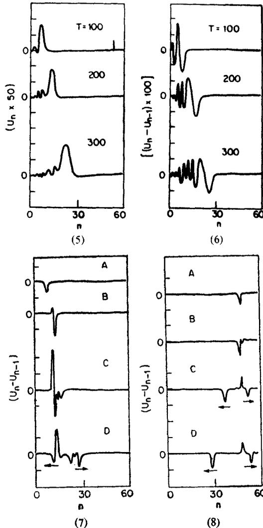
Figures 5-8. 5. Displacement vs atom number. Parameters  $F_0 = 1000.0$ ;  $\beta = 3 \times 3.333$ ;  $k = 0.333$ . 6. Relative displacement vs atom number. Parameters same as for figure 5. 7. The case of a vacancy at the place of 13th atom. Parameters  $F_0 = 3 \times 10^4$ ;  $\beta \times 3.333$ ;  $k = 0.333$ . 8. The case of crossing of an excited atom by a soliton. A backward moving soliton crosses the 48th atom which is just excited. X axis 1 cm = 10 atoms, Y axis = 1 Å
