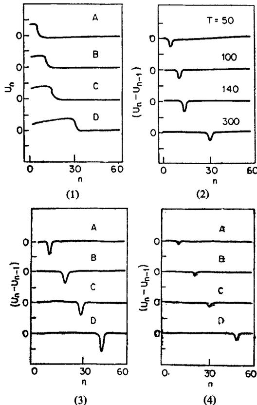
Figures 1-4. 1. Displacement vs atom number. Parameters  $F_0 = 2 \times 10^4$ ,  $\beta = 3.333$ ;  $k = 0.3$ ;  $T = 50$  (for A), 100 (for B); 140 (for C) and 300 (for D). 2. Relative displacement vs atom number. Parameters same as that for figure 1. 3. Parameters  $F_0 = 5 \times 10^4$ ;  $\beta = 3.333$ ;  $k = 0.3$ . 4. Parameters  $F_0 = 2 \times 10^4$ ;  $\beta = 2 \times 3.333$ ;  $k = 0.3$ . X axis 1 cm = 10 atoms, Y axis = 1 Å
