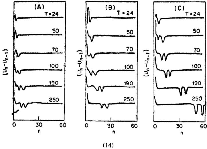
Figures 12-14. 12. The trail left by the soliton in the denser medium as it passes from denser to rarer medium. 13. Crossing of soliton through a defect mass placed at the 30th place. The defect mass is taken as  $m/2$  where  $m$  is the mass of every other atom except the 30th. 14. A.  $u_1 = 0.5$  at  $t = 0$ ; B.  $u_1 = 0.75$  at  $t = 0$ ; C.  $u_1 = 1.0$  at  $t = 0$ . X axis 1 cm = 10 atoms, Y axis = 1 Å
