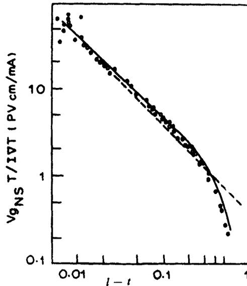
Figure 1.  $V g_{\text{NS}} T / I \cdot \nabla T$  vs  $(1 - t)$ , where  $t = T/T_c$  for sample § 4 of Clarke *et al* (1979a). (•) represents experimental data, (---) has a slope of  $-1$ , (—) is equation 23 fitted at one point.
