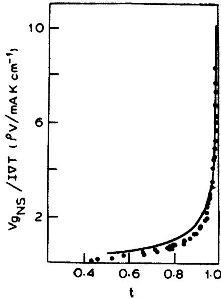
Figure 2.  $Vg_{NS}/T \cdot \nabla T$  vs reduced temperature. (—) represents equation (23) and (•) are the experimental data for sample § 4 of Clarke *et al* (1979a).
