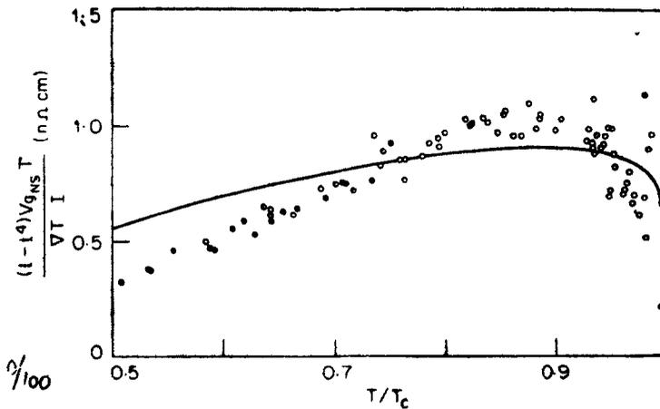
Figure 3. Comparison of theoretical and experimental values of  $(1-t^4) Vg_{NS} T/I \cdot \nabla T$  for sample § 3 of Fjordboge *et al* (1981). The factor  $(1-t^4)$  is included to remove most rapid temperature dependence.
