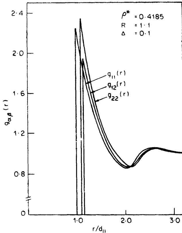
Figure 4. The RDF  $g_{\alpha\beta}(r)$  for a binary mixture of non-additive hard-discs with  $X_1 = X_2 = 0.5$  and  $R = 1.1$  for  $\rho^* = 0.4185$  at  $\Delta = 0.1$ .
