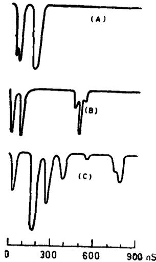
Figure 2. C. R. O. patterns of X-rays A. Only primary focus formed occurrence 35% B: Primary and auxiliary focus occurrence 60% C: Multiple focus formation occurrence 5%.
