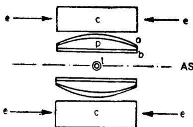
Figure 1. Two dimensional driver: Spherical fusion target,  $t$ , or other payload to be compressed by a cylindrically symmetric liner composed of ablator  $a$ , pusher  $p$  and buffer  $b$ . AS is the axis of symmetry and  $C$  is a preformed annular plasma heated by electron beams  $e$ . An axial magnetic guide field *may* be employed.
