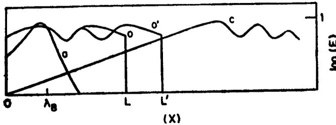
Figure 2. Typical spatial wave energy profiles for absolute instability  $a$ , convective instability  $c$  and two oscillating instabilities  $O$  and  $O'$  corresponding to plasma lengths  $L$  and  $L'$  respectively.
