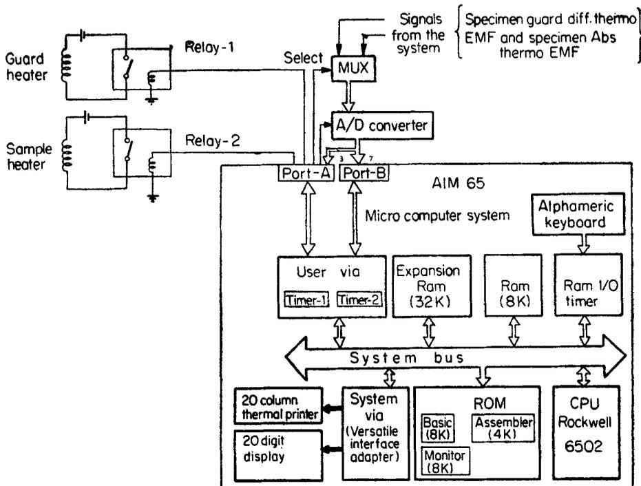
Figure 3. Block diagram of the microcomputer.
