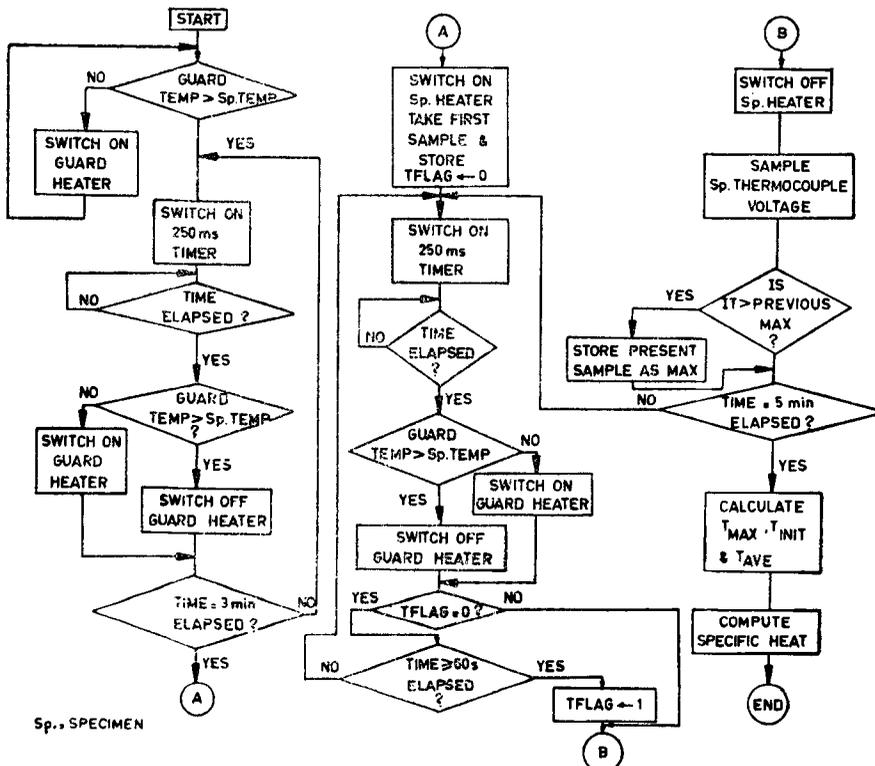
Figure 4. Software for the operation of the microcomputer.
