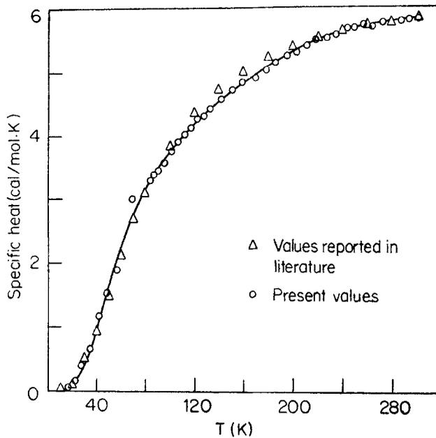
Figure 6. Temperature variation of specific heat for pure copper.
