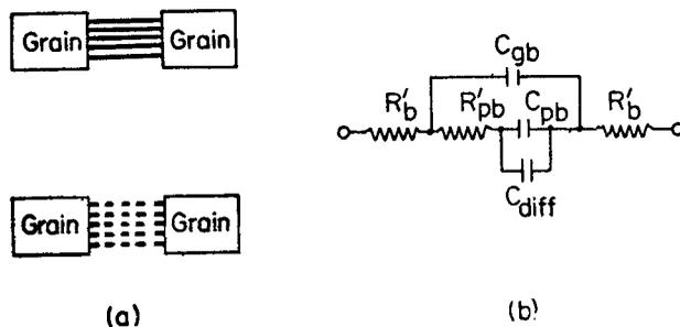
Figure 4. Bridge path model.  $R'_b$ —grain resistance,  $R'_{pb}$ —fraction of bridge path resistance,  $C_{gb}$ —grain boundary capacitance,  $C_{pb}$ —bridge path capacitance,  $C_{diff}$ —diffusion capacitance.
