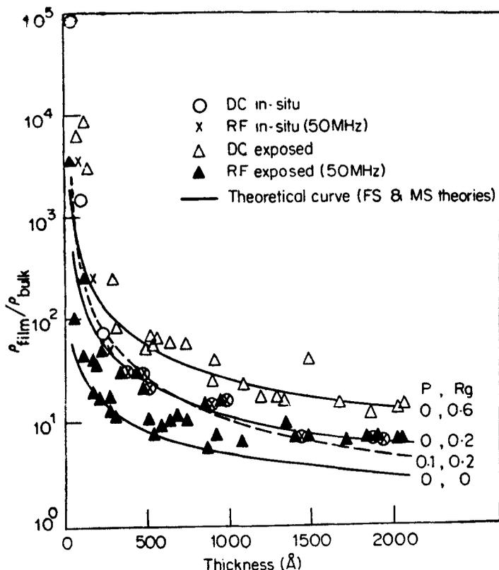
Figure 1. Ratio of film resistivity to bulk resistivity ( $\rho_0 = 1.20 \times 10^{-6}$  mhos-metre) versus thickness under various conditions. RF *in-situ* and RF exposed are co-incident but exposed points ( $\blacktriangle$ ) are shown by the side for convenience.
