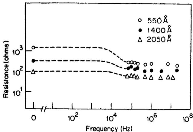
Figure 2. Resistance frequency behaviour of exposed continuous films ( $t > 350 \text{ \AA}$ ) for different thicknesses.
