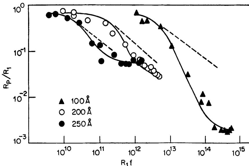
Figure 3. Resistance frequency behaviour (normalized following Humphrey) of exposed discontinuous films ( $t < 350 \text{ \AA}$ ) for different thicknesses.
