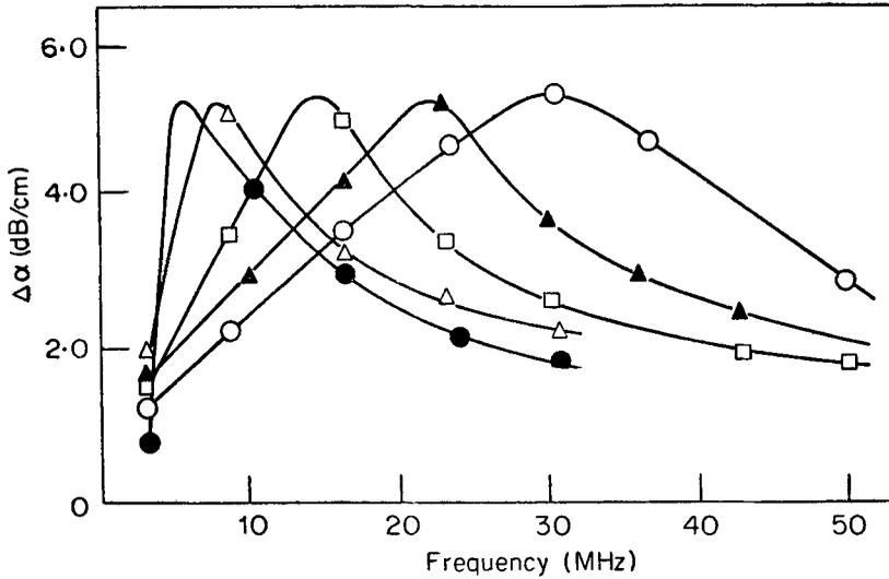
Figure 1. Frequency dependence of  $\Delta\alpha$  at different dislocation densities  $\Lambda$  ( $\Lambda$ 's in  $10^5 \text{ cm}^{-2}$  are given in brackets) ● (0.01); △ (0.06); □ (2.00); ▲ (20.00); ○ (110.00).
