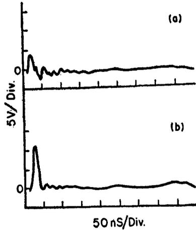
Figure 3a. Faraday cup signal for intense beam propagation in vacuum. b. Faraday cup output with a conditioned 5.0 cm diameter perspex tube as a beam guide.
