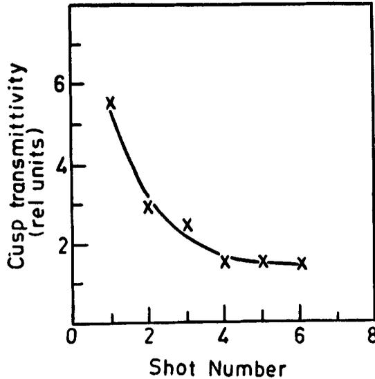
Figure 4. Variation of the cusp transmittivity with shot number after the pumpdown from atmospheric pressure. Diameter of the perspex tube used is 5 cm.
