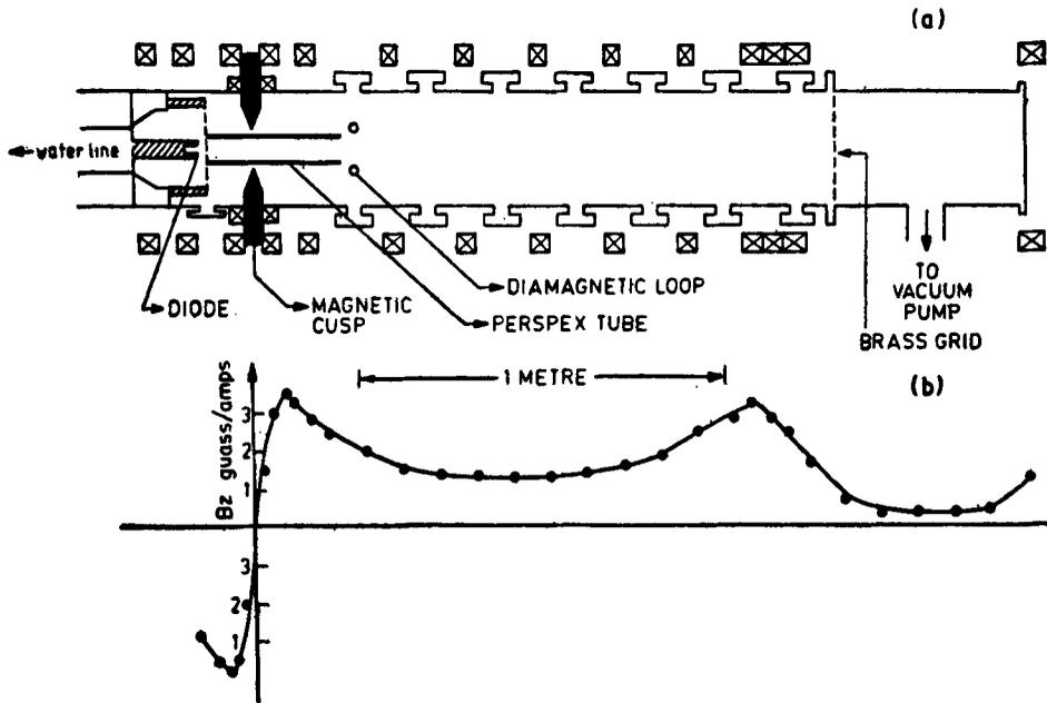
Figure 1. a. Schematic drawing of the experimental system. b. External magnetic field configuration.
