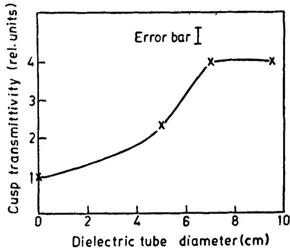
Figure 5. Variation of the diamagnetic loop output with perspex guide tube diameter. B mirror = 650 gauss. In all the cases the tube was conditioned with a number of shots.
