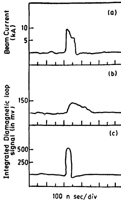
Figure 2. a. Diode current signal measured using a self-integrated Rogowskii Coil. b. Diamagnetic signal for beam propagated in vacuum. c. Diamagnetic loop output for beam propagation using 5.0 cm diameter perspex tube.
