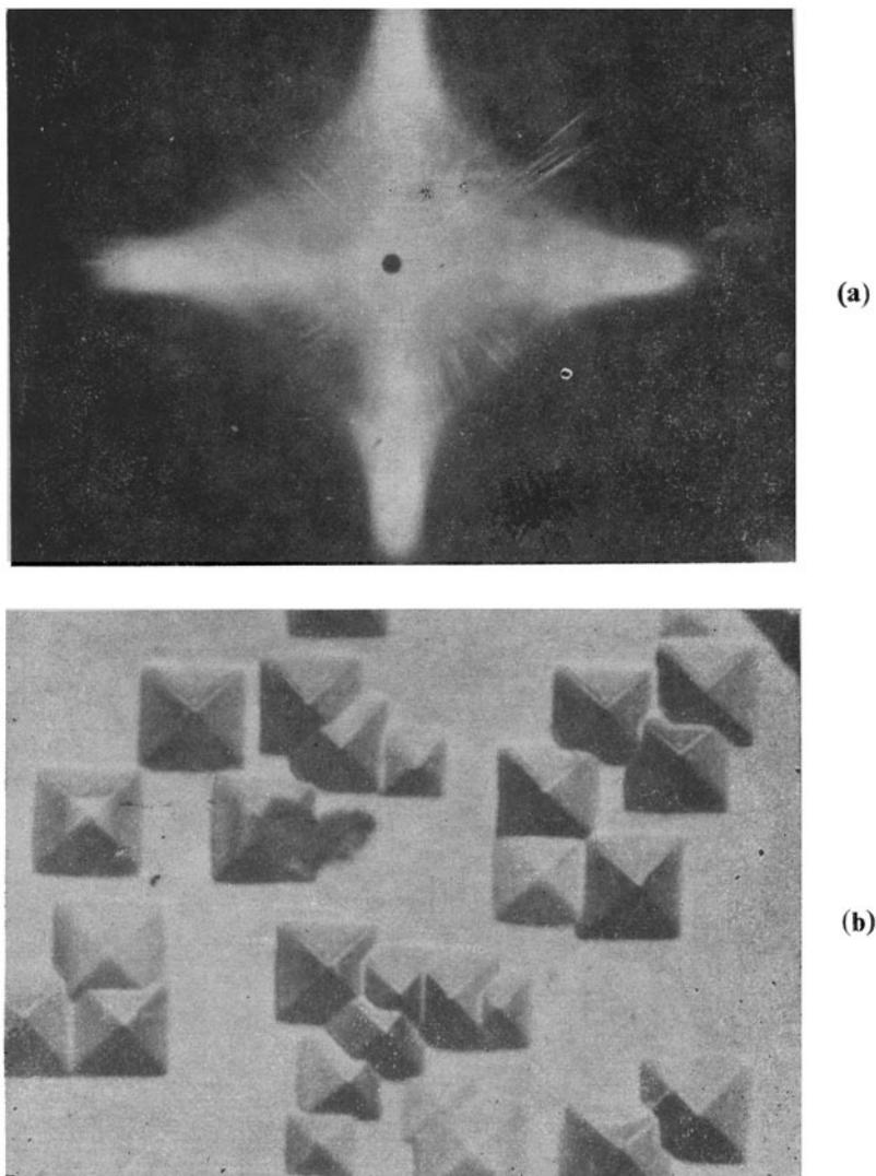
**Figure 4.** Square pits with edges parallel to  $\langle 100 \rangle$  direction. Poison concentration:  $4 \times 10^{-4}$  mg/cc. Etching time: 15 min. a. Optical topograph. b. etched and silvered faces ( $\times 1200$ )
