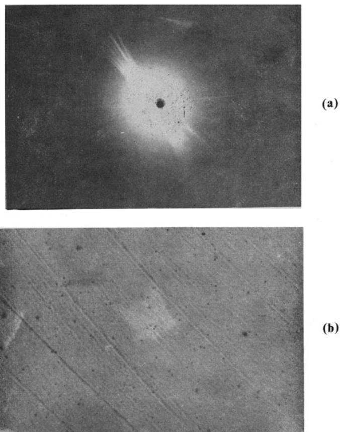
**Figure 10.** Etched surface. Poison concentration  $4 \times 10^{-4}$  mg/cc. Etching time: 6 min. **a.** Optical topograph. **b.** etched and silvered faces ( $\times 300$ ).
