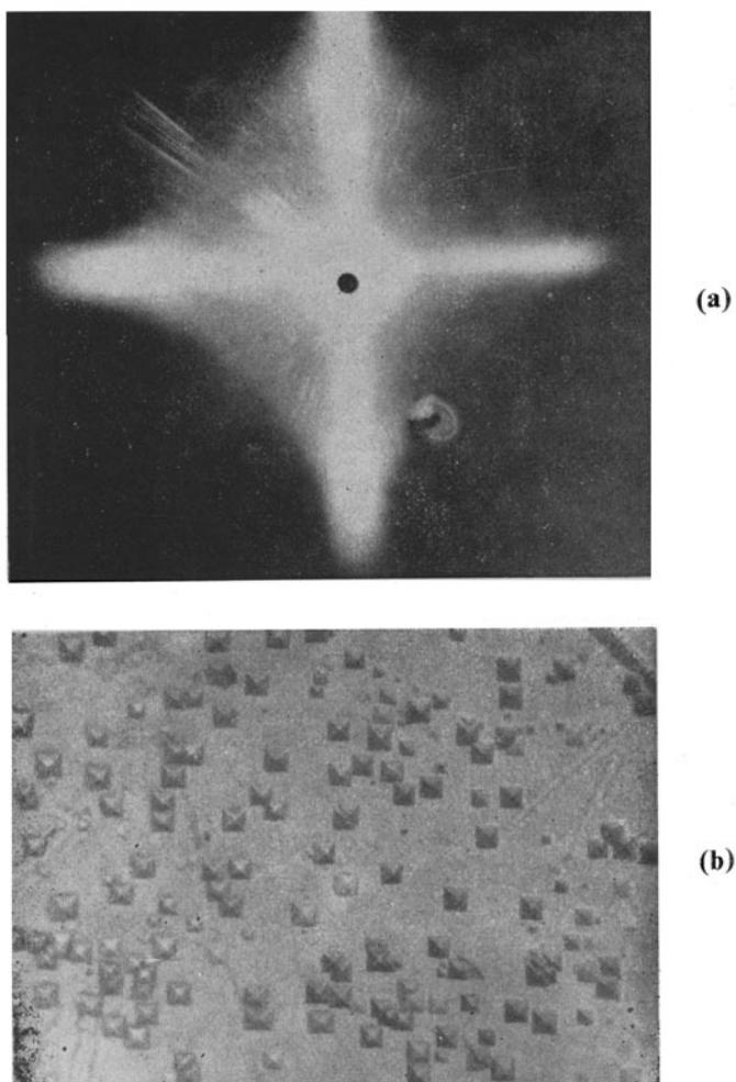
**Figure 12.** Square pits with edges parallel to  $\langle 100 \rangle$  direction. Poison concentration:  $4 \times 10^{-4}$  mg/cc. Etching time: 15 min. a. Optical topograph. b. Etched and silvered faces ( $\times 300$ ).
