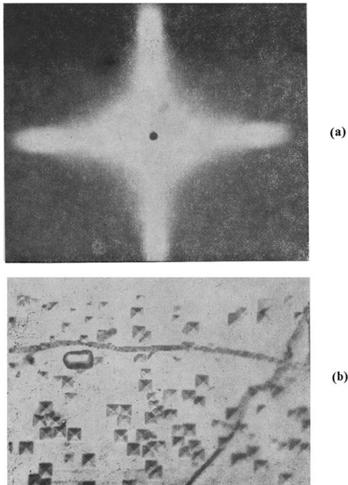
**Figure 13.** Square pits with edges parallel, to  $\langle 100 \rangle$  direction. Poison concentration:  $4 \times 10^{-4}$  mg/cc. Etching time: 20 min. a. Optical topograph. b. Etched and silvered faces ( $\times 300$ ).
