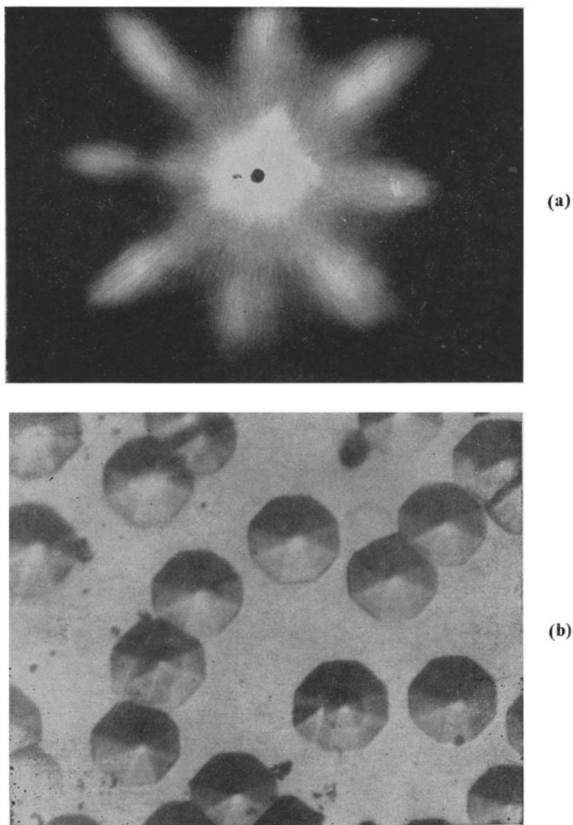
**Figure 6.** Octagonal pits with edges parallel to  $\langle 110 \rangle$  direction greater than that of  $\langle 100 \rangle$  direction. Poison concentration:  $4 \times 10^{-3}$  mg/cc. Etching time: 15 min. **a.** Optical topograph. **b.** etched and silvered faces ( $\times 1200$ ).
