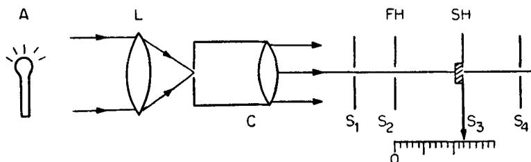
Figure 1. Experimental arrangement. A. light source. L. the lens. C. collimator.  $S_1$  circular slit. PH photographic film holder. SH sample holder.
