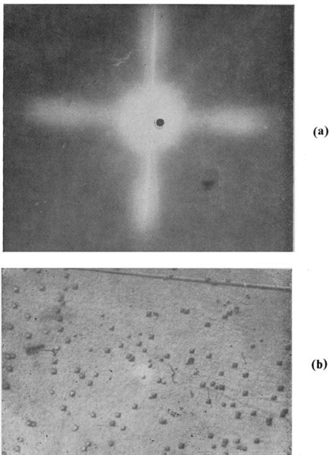
**Figure 11.** Pits with edges parallel to  $\langle 100 \rangle$  direction. Poison concentration:  $4 \times 10^{-4}$  mg/cc. Etching time: 10 min. **a.** Optical topograph. **b.** Etched and silvered faces ( $\times 300$ ).
