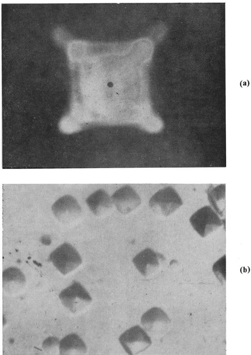
**Figure 7.** Square pits with edges parallel to  $\langle 110 \rangle$  direction. Poison concentration  $1 \times 10^{-1}$  mg/cc. Etching time: 15 min. a. Optical topograph. b. etched and silvered faces ( $\times 1200$ ).
