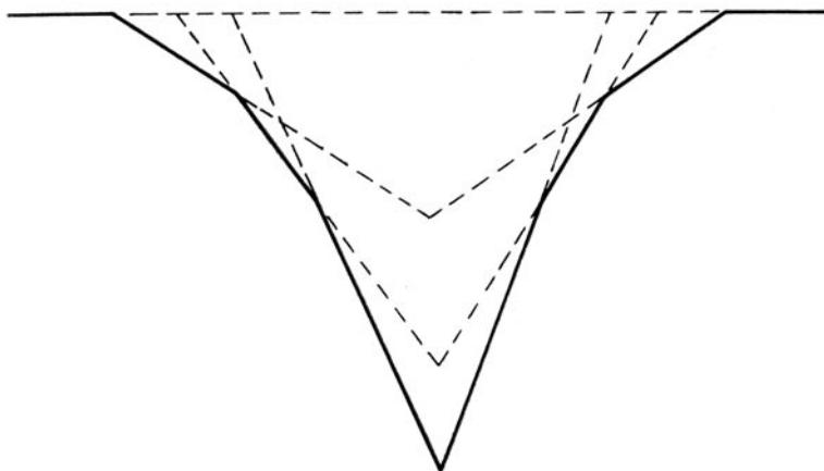
**Figure 8.** A vertical section of an etch pit illustrating the nature of the surface forming the pit sides.
