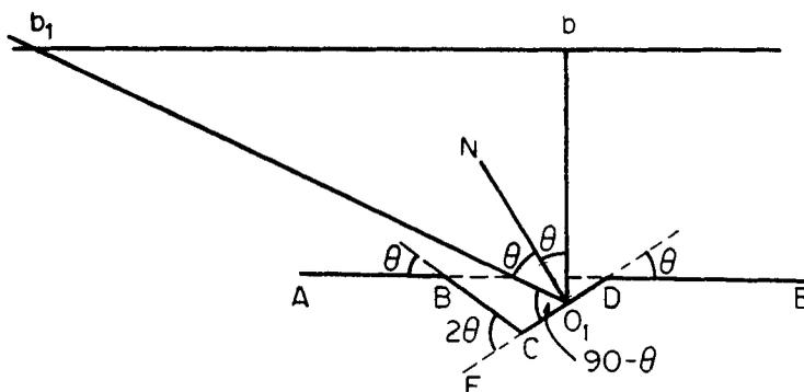
Figure 3. Vertical section of an etch pit.
