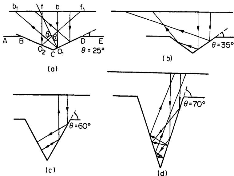
Figure 2. a-d. A vertical section of an etched surface showing pits of different inclinations and the reflected beams.
