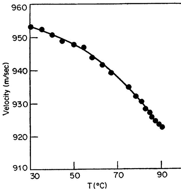
Figure 4. Transverse wave velocity in amorphous  $\text{Ge}_{10}\text{Se}_{90}$  sample plotted against temperature.
