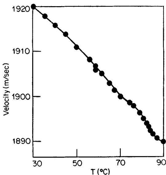
Figure 3. Longitudinal wave velocity in amorphous  $\text{Ge}_{10}\text{Se}_{90}$  sample plotted against temperature.
