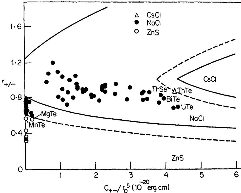
Figure 3. Areas of stability of the CsCl, NaCl and ZnS structures among divalent AB crystals in the  $(r_{+/-})$  vs  $(c_{+-}/r_0^5)$  plane. The solid lines are given by theory while the dashed lines have been empirically drawn for perfect separation of the observed structures.
