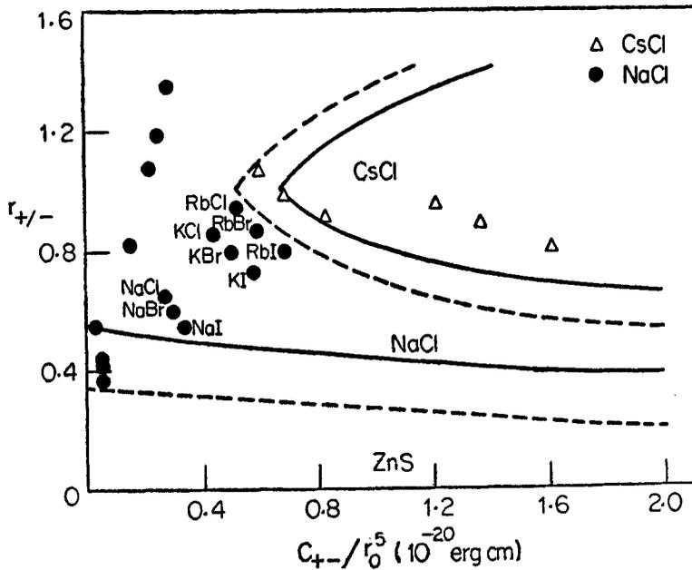
Figure 2. Areas of stability of the CsCl, NaCl and ZnS structures among monovalent AB crystals in the  $(r_{+/-})$  vs  $(c_{+-}/r_0^5)$  plane. The solid lines are given by theory while the dashed lines have been empirically drawn for perfect separation of the observed structures.
