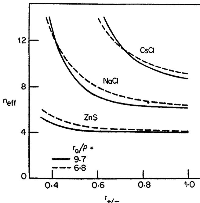
Figure 1. Variation of the effective number of neighbours with the radius ratio in the CsCl, NaCl and ZnS structures. The solid lines correspond to monovalent crystals ( $A^+ B^-$ ) with  $r_0/\rho = 9.7$  and the dashed lines to divalent crystals ( $A^{2+} B^{2-}$ ) with  $r_0/\rho = 6.8$ .
