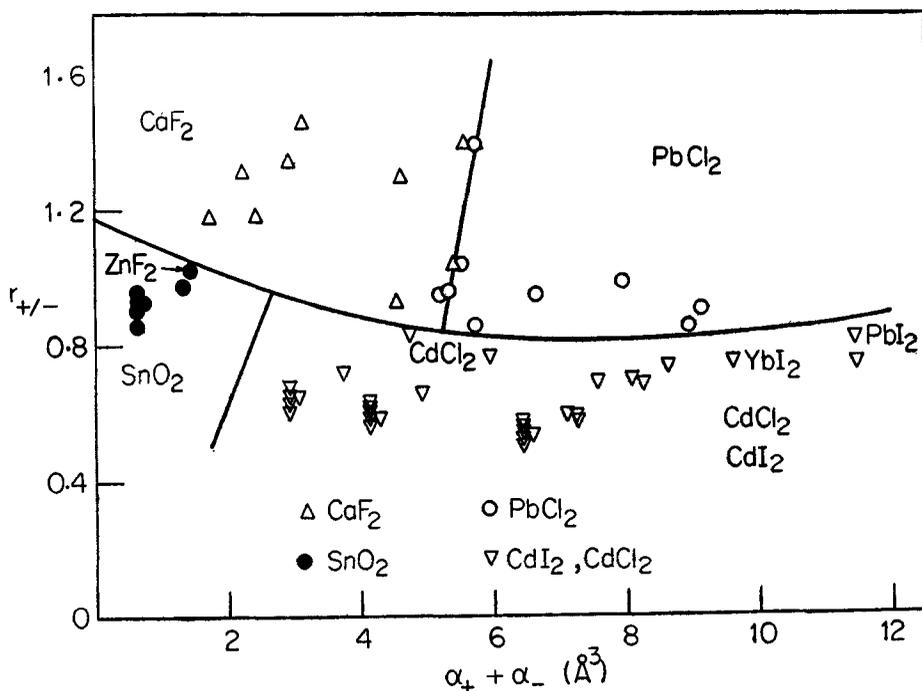
**Figure 4.** Areas of stability of the  $\text{CaF}_2$ ,  $\text{PbCl}_2$ ,  $\text{SnO}_2$  and  $\text{CdI}_2$  ( $\text{CdCl}_2$ ) structures among  $A^2+B_2$  halides. The separating lines have been drawn empirically.
