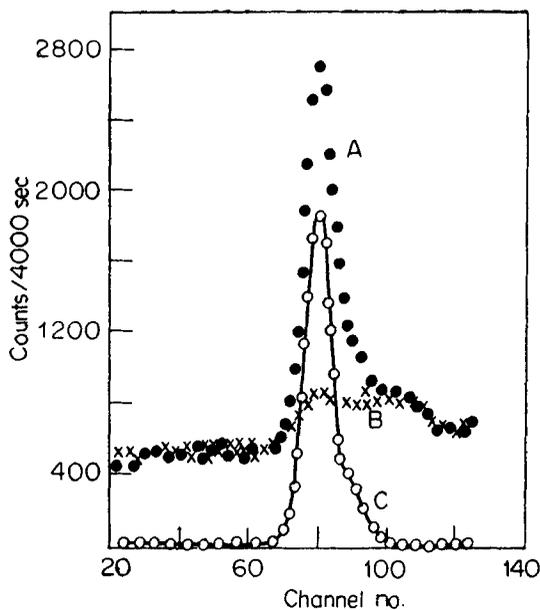
Figure 2. Comparison target spectra recorded with proportional counter spectrometer. A—Rb primary and Se comparison. B—Eq. A1 primary and Se comparison. C—K x-rays of Se ( $=A-B$ ). Only representative data points are shown on different curves for the sake of clarity.
