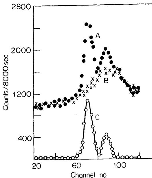
Figure 1. Secondary target spectra recorded with proportional counter spectrometer. A—Rb primary and Pb secondary. B—Eq. A1 primary and Pb secondary. C— $L_{III}$  x-rays of Pb ( $=A-B$ ). Only the representative data points are shown on different curves for the sake of clarity.
