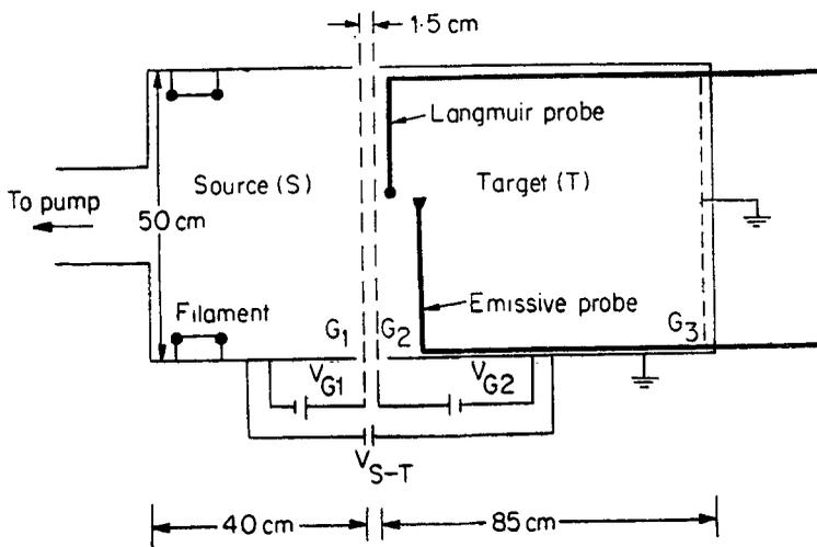
Figure 1. Schematics of the double plasma device. Drifting electrons are produced by biasing the source chamber negative with respect to the target chamber. Grid G1 is biased 0 V with respect to the source, potential of the grid G2 is varied between 0–20 V with respect to the ground, and G3 is grounded.
