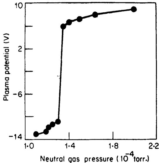
Figure 4. The plasma potential at 10 cm from the grid G2 is plotted for various neutral gas pressures. The device control settings are  $G1 = 0$  V,  $G2 = 10$  V,  $G3$  is grounded  $V_{S-T} = -8.3$  V. Note the sharp transition in the plasma potential between  $1.3 - 1.35 \times 10^{-4}$  torr.
