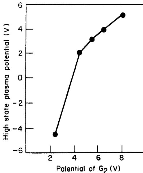
Figure 3. A plot between the high-state potential and the potential of the grid G2.
