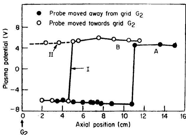
Figure 2. The plasma potential is plotted for various axial positions of the emissive probe. Profile A corresponds to when the emissive probe is moved away from the grid G2 and profile B when the emissive probe is moved towards the grid G2. The dashed line (branch II of the profile B) shows that occasionally the entire plasma remains at high-potential state.
