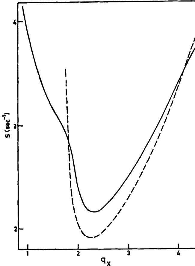
Figure 1. Neutral stability curves for RI in shear flow for HBAB. The dashed curve has been calculated from equation (11).
