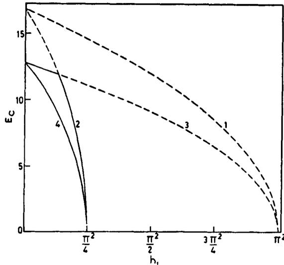
Figure 5. Variation of critical Ericksen number  $E_c$  of HI with destabilizing field in plane Poiseuille flow of MBBA.  $E_c$  as a function of  $h_3 = (\Delta\chi)H_3^2 a^2/K_{33}$ ; curve (1) for splay mode; curve (4) for twist mode.  $E_c$  as a function of  $h_1 = (\Delta\chi)H_1^2 a^2/K_{11}$ ; curve (2) for splay mode; curve (3) for twist mode. Dashed portions of the curves are of only theoretical interest.
