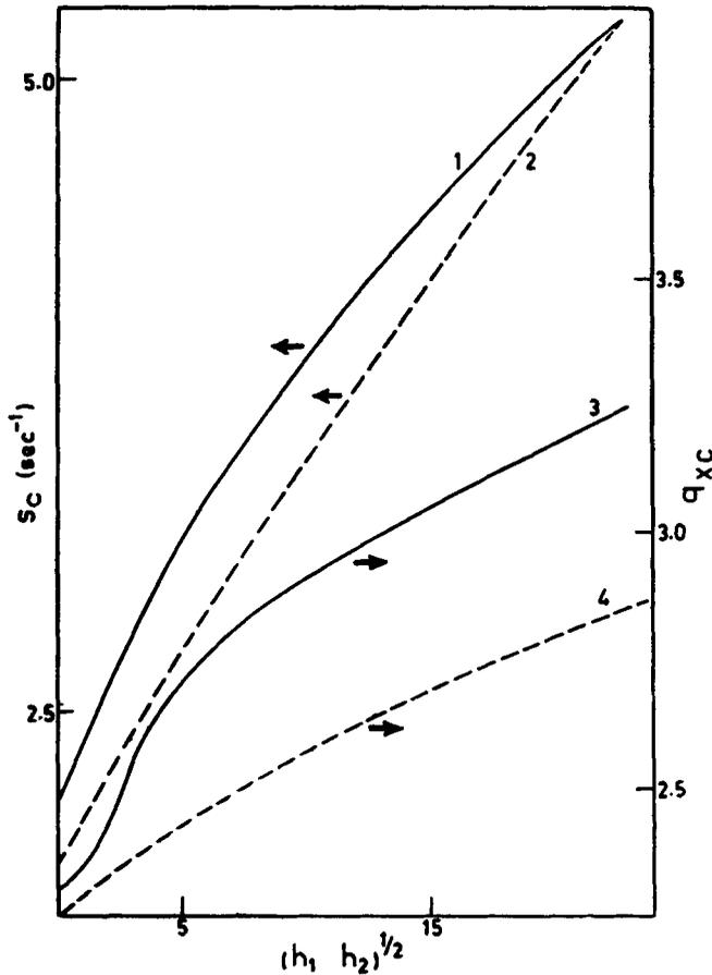
Figure 2. RI threshold  $S_c$  (curves 1 and 2) critical wave vector  $q_{xc}$  (curves 3 and 4) as functions of  $(h_1, h_2)^{1/2} = (\Delta\chi)H_3^2 a^2 / (K_{11}K_{22})^{1/2}$  for HBAB. Full and dashed curves are respectively from the exact calculation and equation (11).
