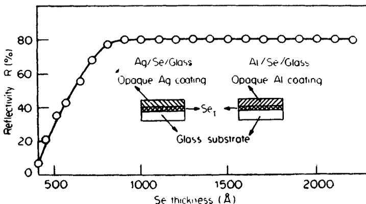
Figure 2. Variation of reflectivity with Se thickness overcoated with opaque Ag layer at  $\lambda$  5461 Å.
