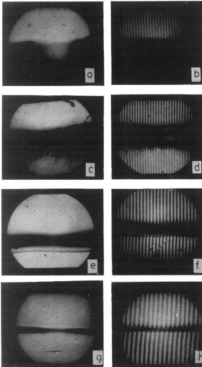
**Figure 4.** Appearance of diffusion area as formed by Linnik microscope as well as two-beam interference fringes with diffusion area for Se film overcoated with Ag. **a** and **b**. Film thickness 230 Å. **c** and **d**. 800 Å. **e** and **f**. 977 Å. **g** and **h**. 1600 Å.
