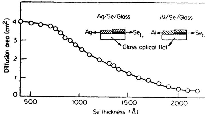
Figure 5. Variation of diffusion area with Se thickness overcoated with opaque Ag layer.
