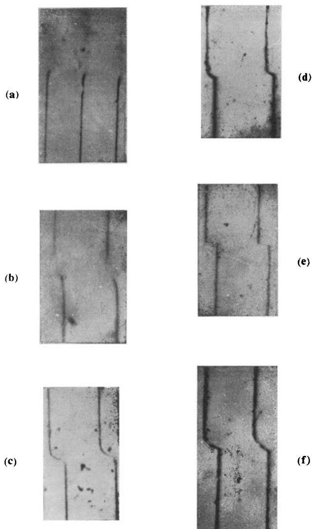
**Figure 3.** a and b. Appearance of multiple beam fringes at reflection for Se layer of thickness 230 Å overcoated with opaque layers of Ag and Al respectively. c and d. Layer thickness 655Å. e and f. Layer thickness 908 Å.
