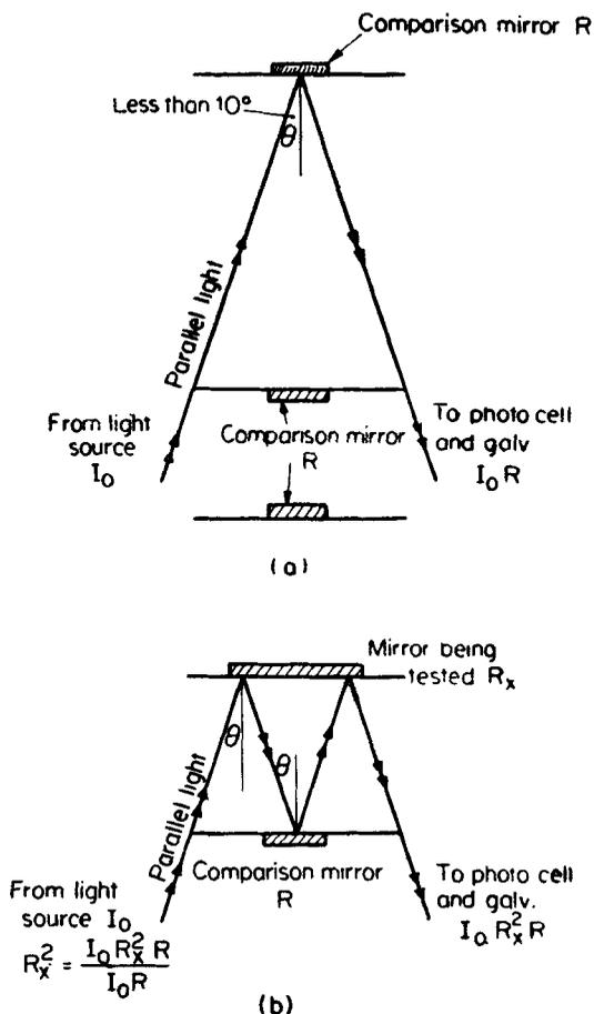
Figure 1. Optical system for reflectivity measurement.
