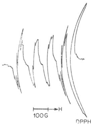
Figure 1. ESR spectra of \text{Cu}^{2+} ion in TGCB at 20^\circ to a axis in ac plane.
