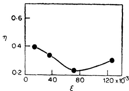
Figure 10. Reflection coefficient as a function of the adiabaticity parameter for the plasma case.
