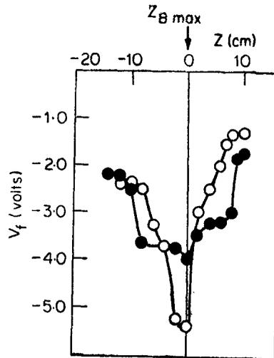
Figure 11. Axial floating potential profile around the mirror point for III and V magnetic field configurations during the plasma experiments.
