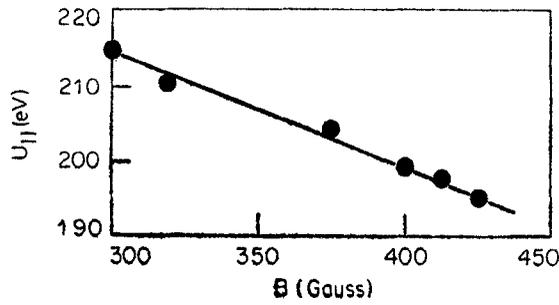
Figure 4. Parallel energy of the electrons as a function of the axial magnetic field.
