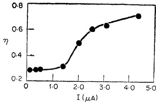
Figure 12. Dependence of the reflection coefficient on the beam current  $I$  for the electron beam.
