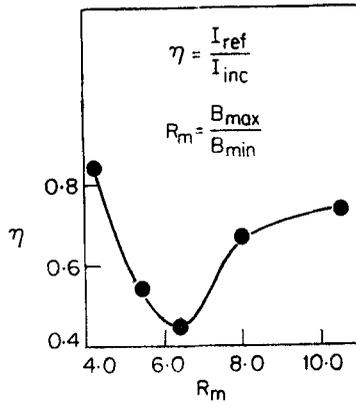
Figure 5. Dependence of the reflection coefficient ( $\eta$ ) on the mirror ratio ( $R_m$ ).
