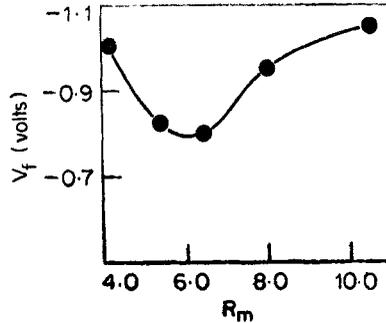
Figure 7. Floating potential at the centre of the system as a function of mirror ratio.
