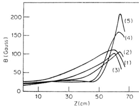
Figure 2. Axial magnetic field distribution from centre of the system to one of the mirrors for five different mirror configurations.
