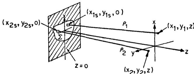
Figure 2. Geometry for calculating the temporal Fourier transform  $\hat{\Gamma}$  in the plane  $z$ .
