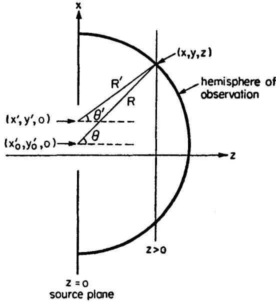
Figure 1. Geometry of the diffraction problem and the hemisphere of observation.
