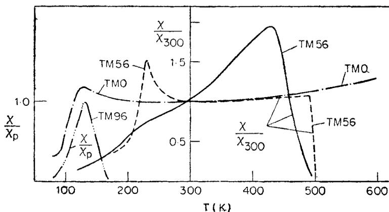
Figure 3. Susceptibility-temperature curves for the synthetic samples. TM0- $\text{Fe}_3\text{O}_4$ ; TM56- $0.44\text{Fe}_3\text{O}_4 \cdot 0.56\text{Fe}_2\text{TiO}_4$ ; TM96- $0.04\text{Fe}_3\text{O}_4 \cdot 0.96\text{Fe}_2\text{TiO}_4$ .
