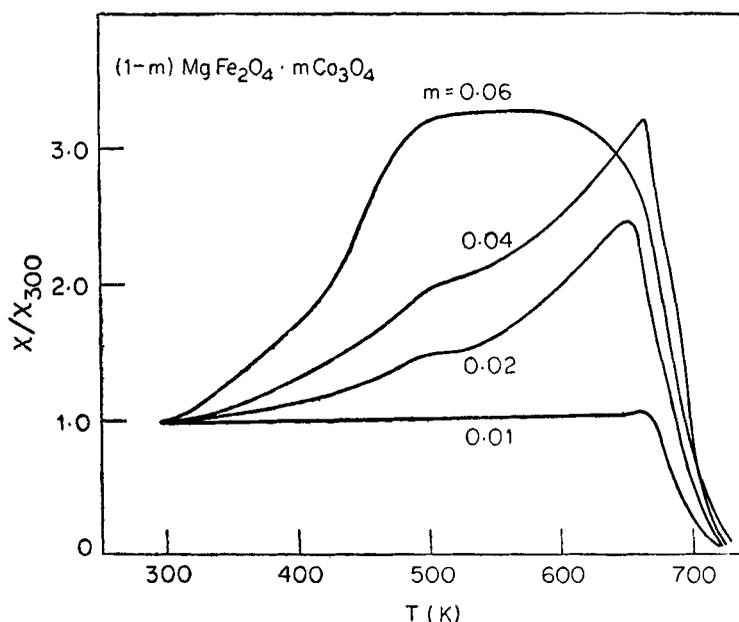
**Figure 4.** Susceptibility-temperature curves for the samples of the series  $(1-m)\text{MgFe}_2\text{O}_4 \cdot m\text{Co}_3\text{O}_4$  for  $m=0.01$ ,  $0.02$ ,  $0.04$  and  $0.06$ .
