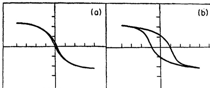
Figure 1. Hysteresis loops obtained in a peak field of 1500 Oe for a. a piece of natural magnetite ore and b. a small quantity of commercial magnetite powder having acicular SD particles,
