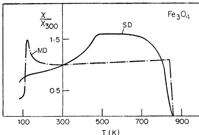
Figure 2. Susceptibility-temperature curves for the magnetite samples of figure 1.
