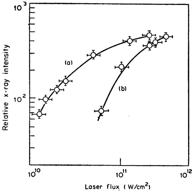
Figure 7. Variation of x-ray intensity with laser flux for carbon (A) and polyethylene (B).
