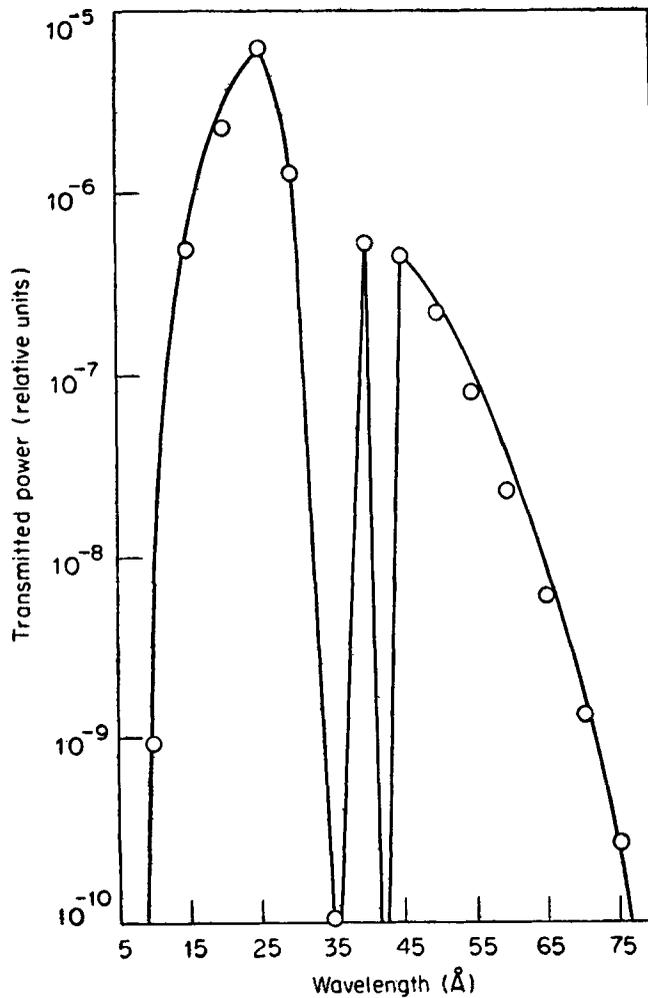
Figure 3a. Spectral profile of transmitted radiation through two B-10 foils at 50 eV
