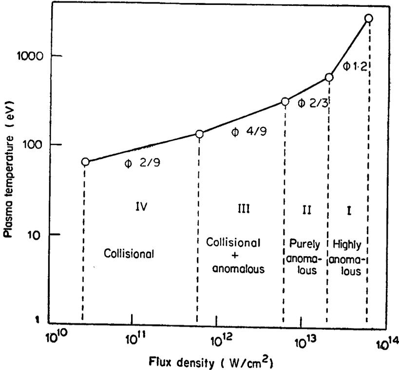
Figure 9. A tentative schematic diagram of the scaling law of plasma temperature against flux.
