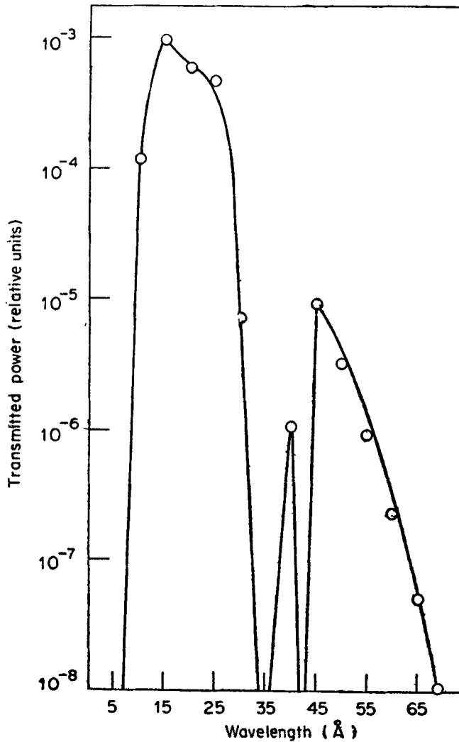
Figure 3b. Spectral profile of transmitted radiation through two B-10 foils at 100 eV.
