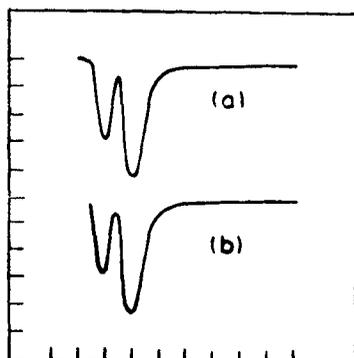
Figure 4. Oscilloscope trace of successive laser and x-ray pulse for a polyethylene plasma.
