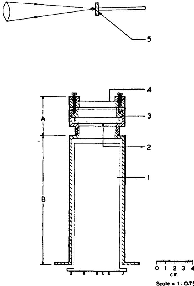
Figure 1. Experimental set up with scintillator detector assembly.
