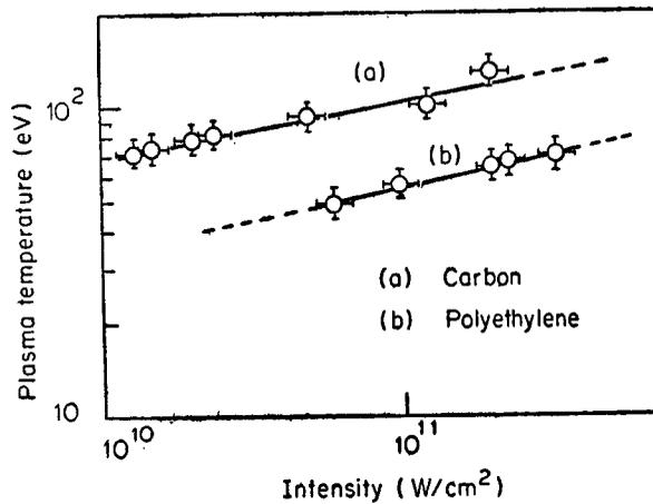
Figure 8. Variation of plasma temperature with flux for carbon (A) and polyethylene (B).
