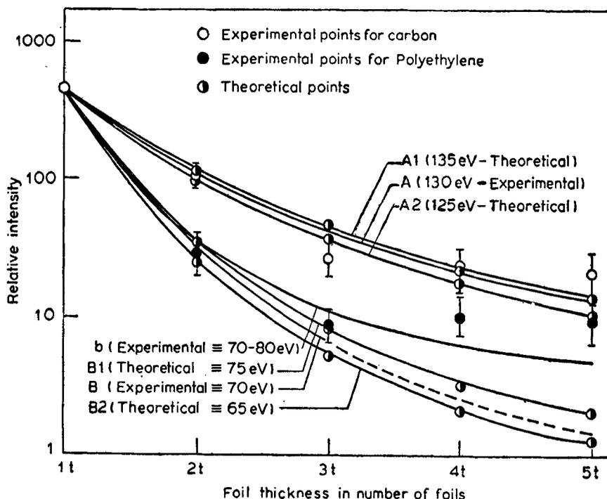
Figure 6. Variation of relative x-ray intensity with number of foils. A for carbon, B for polyethylene.
