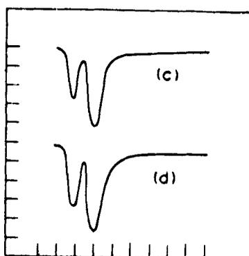
Figure 5. Oscilloscope trace of successive laser and x-ray pulse for a polyethylene plasma.
