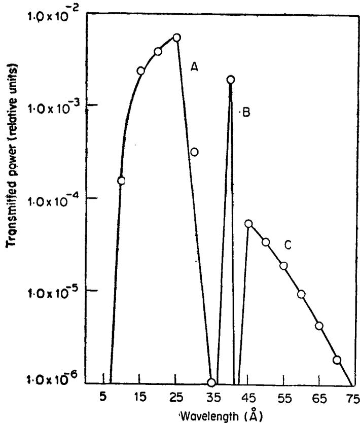
Figure 2b. Spectral profile of transmitted radiation through one B-10 foil at 100 eV.
