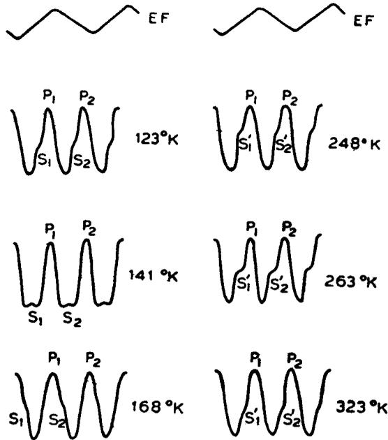
Figure 3. Brightness waves of ZnO:Nd electroluminor at different temperatures ( $V = 500 \text{ V}$ ;  $f = 500 \text{ Hz}$ )
