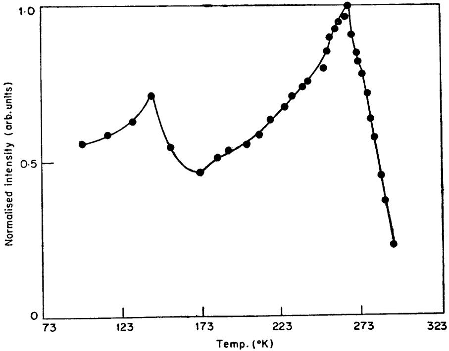
Figure 4. Temperature dependence of EL output for ZnO:Nd electroluminor ( $f = 500 \text{ Hz}$ ;  $V = 500 \text{ V}$ )
