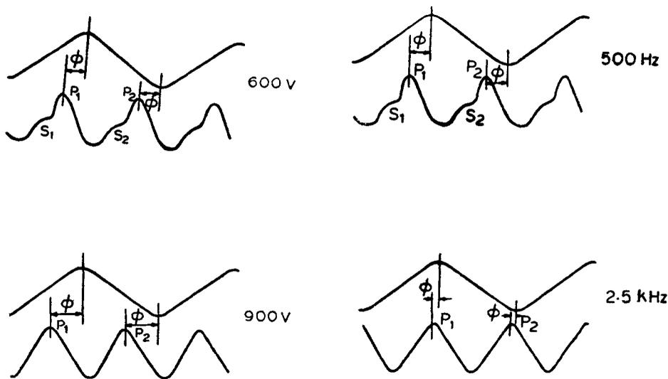
**Figure 1.** Brightness waves of ZnO:Nd electroluminor at different voltages ( $f = 500$  Hz;  $T = 273^\circ\text{K}$ )
